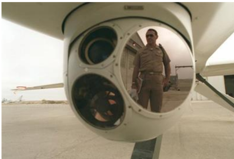
Photo courtesy U.S. Air Force The RQ-1 uses a set of nose cameras to "see" on missions.
