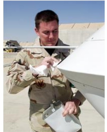
Photo courtesy U.S. Air Force An airman cleans the lens pilots use to fly the MQ-1 Predator.
