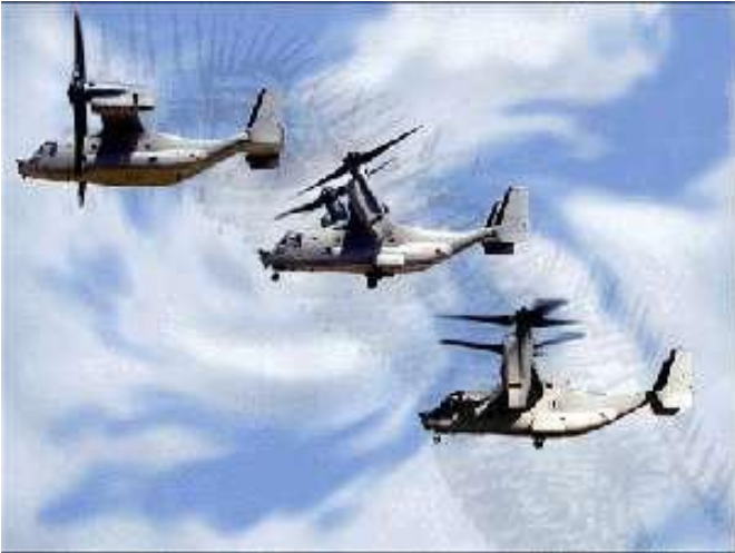
V-22 osprey transitioning from helicopter to airplane mode
