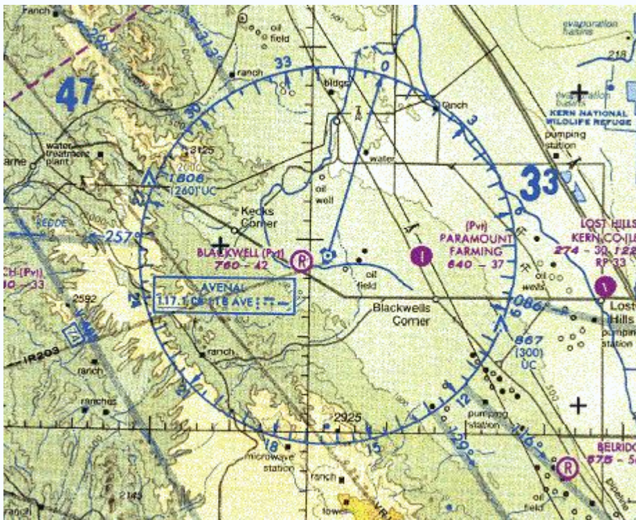
The Avenal VOR shown on a sectional aeronautical chart. Notice the light blue airways radiating from the VOR. (click to enlarge)
