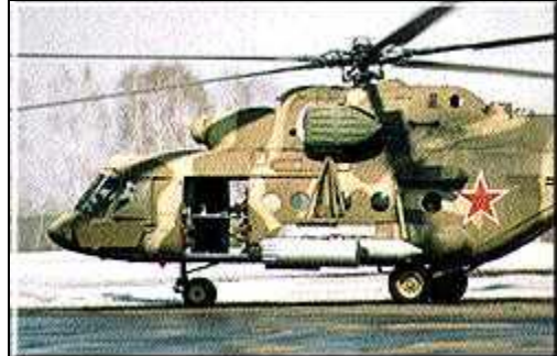
The enlarged port-side sliding door and the unguided rocket pod suspended from the rack
