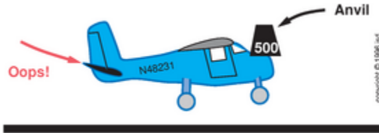
Figure 6.10 : Center of Mass Too Far Forward
