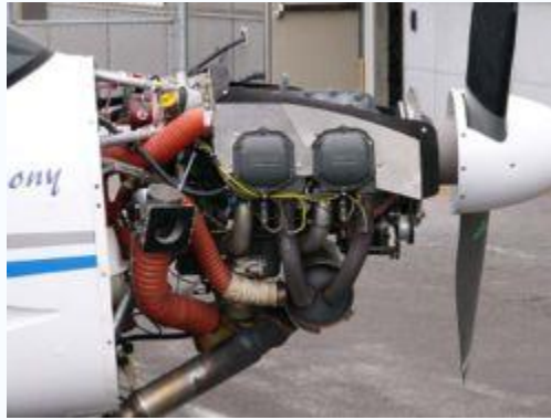
A Lycoming O-320-D2A installed in a Symphony SA-160
