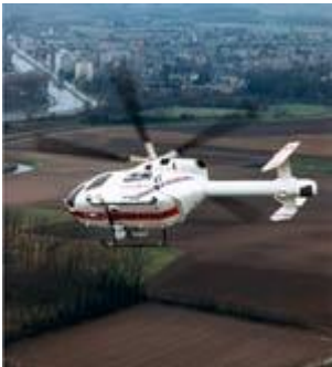
Instead of a tail rotor, the MD Explorer is equipped with the NOTAR anti-torque system.
