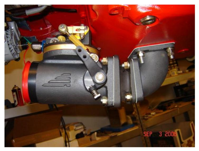
The throttle mechanism is on the left side and the mixture is on the right. Notice in the picture above that there are TWO mounting holes for the cable rod end. The lower hole allows about 2 inches of travel, and the upper hole allows about 2.5 inches of travel.
