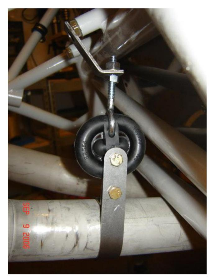
The exhaust hangers were fun to put together. The instructions are pretty basic and straight forward. You have to drill and bend some mild steel to correspond to the angle of the footwell engine mount bolts, then bolt it up. Simple and effective. The pic shows the bracket on the outside of the tailpipe, which puts the two pipe tail end openings quite close together. I don't know if that has any effect on noise or performance, so I'm waiting to hear on that issue, too.
