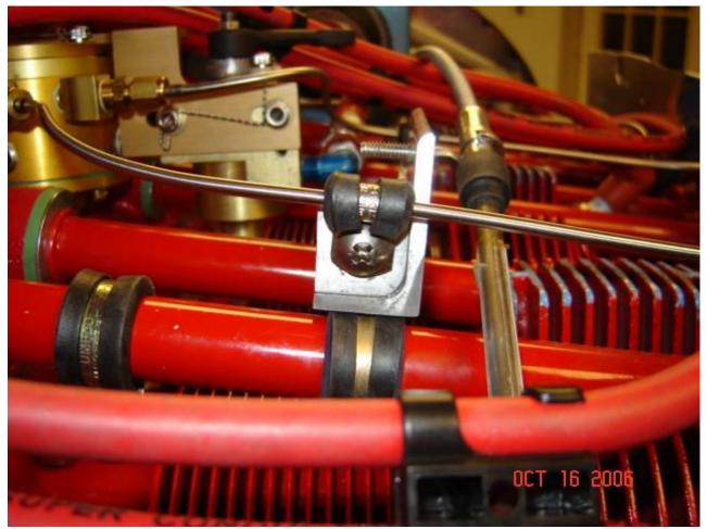
The bracket is held in position on the pushrod tubes by #12 WDG (wedge) Adel clamps. The fuel injection line has an Adel clamp, too. I cut up a piece of 3/4x/34 angle and stuck it to the big cable bracket with one AD4-6 rivet and some JB Weld.
