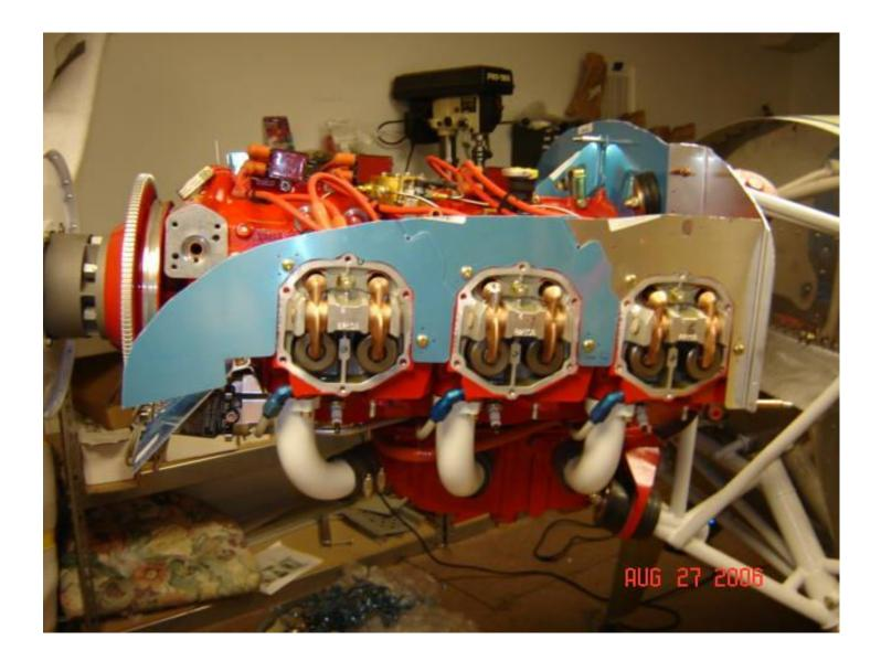
For those of you who are getting a Mattituck TMX engine, or dual Lightspeed Plasma III electronic ignition and fuel injection, the top of the engine gets quite crowded. I had to remove the front sky hook and reposition it to the front boss and move two of the coil sets toward the middle of the engine. I had to move things around in order to fit everything inside the baffles as well as to fit the cowl over the top.
