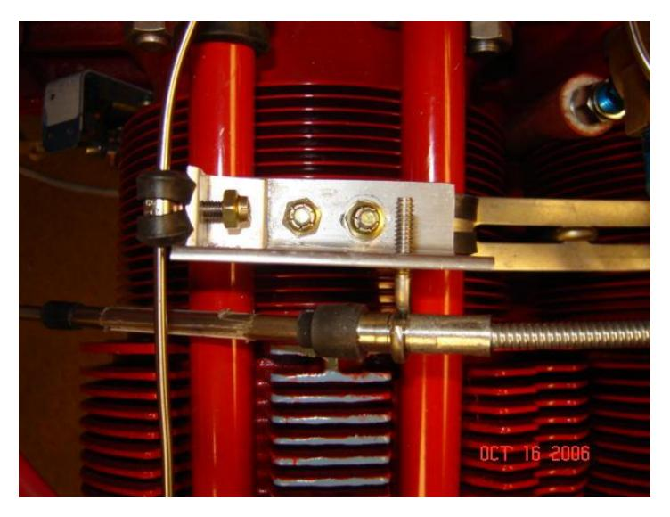
The prop governor cable bracket is just test fitted. It needs to be cut down some that then primed and painted. Also, I'll use a stainless eye bolt that completely contains (retained) the cable, unlike the "hook" in the picture. I might need to attach other cables or wires to the bracket, so I'm leaving it as is until I get a little farther along. Still have to attach the purge valve cable and secure the spark plug wires.
