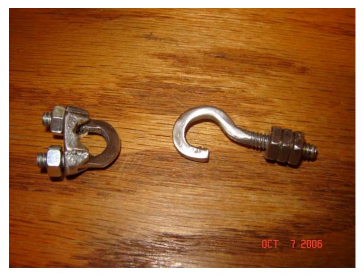
At this point, I'm using the stainless steel eye bolt. I may scrap the idea and remake the entire bracket using only 1/8 angle and safety wire. The stainless eye bolt crimps around the cable quite securely. The problem is that the tension for and aft on the eye bolt in service may tend to loosen up the rather small diameter shank and nuts. Not a good situation. Although in a test fit, the setup seems quite secure. Either way, I'm definitely adding some safety wire.
