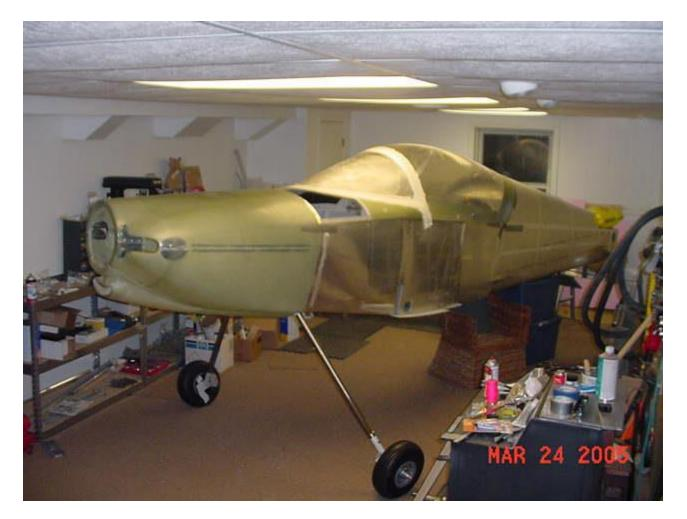
The cowl is stuck on with duct tape. It stays put pretty well that way. But I have it on without bottom support just for this photo op.
