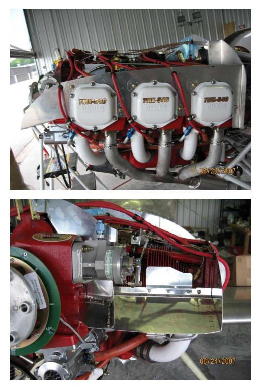
I may insert an air vent duct on the left air ramp scoop above. There's lots of room at the back, and logistically that may be easier. I'll insert that last. The right side is ready for soft baffle. Time to finish up the right side!
