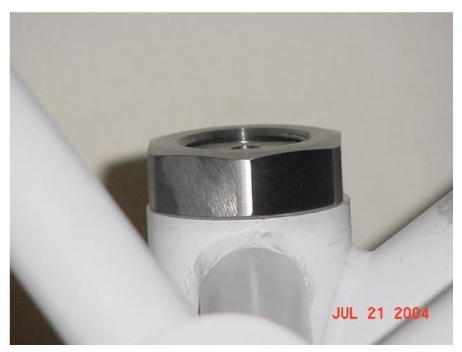
This is as far as the nut goes on the leg after another hour of reaming with Oatley cutting oil and a "breaker bar". I ruined a ratchet doing this little chore. I was really leaning on the reamer, and it was moaning all the way around. It felt like I was really biting into the metal. But this process is much slower, and a lot more work than I ever care to try again. My recommendation: get your EM from Mark and make sure HE reams it for you!
