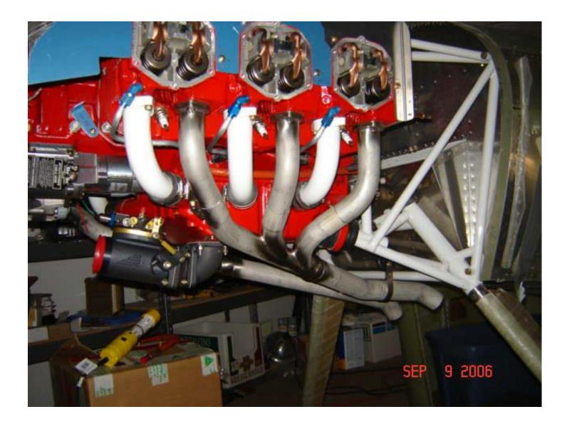
With a test hang of the system, it looks like the tailpipe is going to hang too low into the cowl out of the box. Once the unit was bolted up, it was very easy to relocate the tailpipe by rotating it at the ball joint. The hangers are supposed to hold the tailpipe in position.
