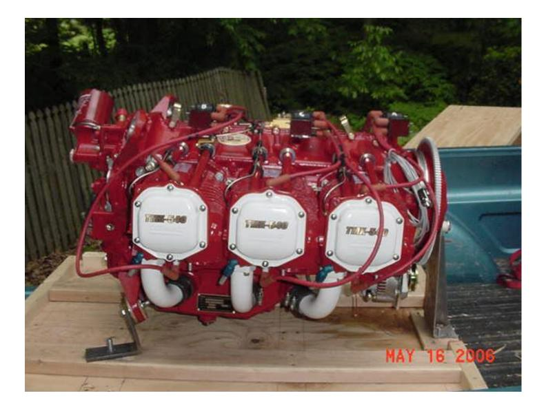
I had wondered how they would mount the engine in the crate. There are custom steel feet that are bolted to the engine and the crate. Very nice. looking over the engine, it sure is a beauty. And it's amazing how complete it is! Now to get it on the hoist and get it inside before it rains. A little tricky to do since I have to take it though my walk through gate, along my winding walkway, and into my basement.
