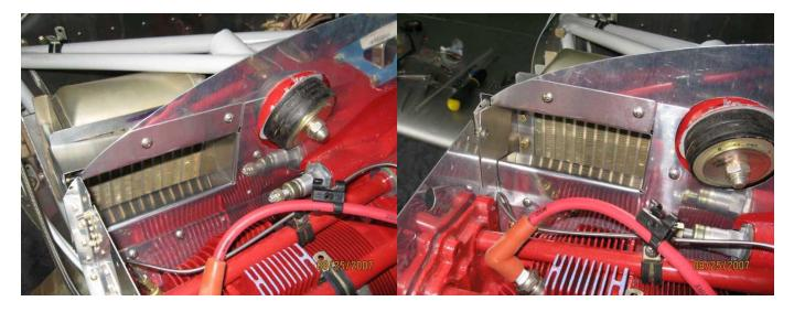
Sorry, no pics of the silicone parts, they just wouldn't show up.There is about 1/4 to 3/8 clearance between the oil cooler duct and the baffle duct. The silicone material is riveted to the outside of the baffle duct flanges so that the silicone material seals between the ducts (of course!).
