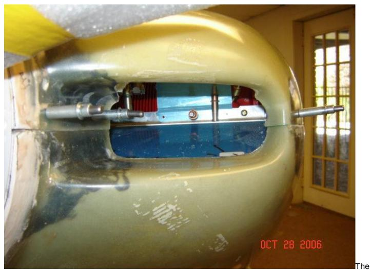
left side inlet ramp has a longer and more gradual angle at the air inlet. I cut the ramp on that one just right. I still may have to cut it back more soon as I decide how I want to transition between the fixed cowling and the movable (shaking with the engine) baffles.
