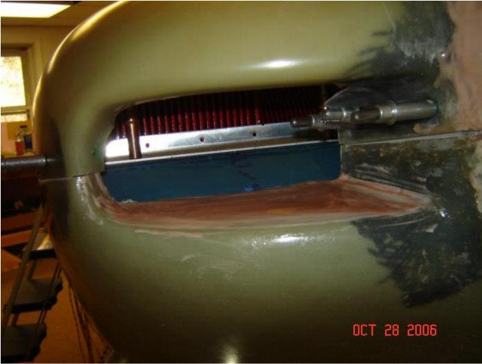
With the aft and side baffles trimmed and dressed to shape, time to go back and work on the front baffles and then start assembling the hard parts. I've already got them nearly roughed out. For me, that means probably a full day or more working on them just to get them to fit.
