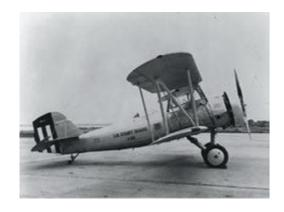
**O2U-2:** version with increased-span upper wing and wing refinements, larger rudder and R-1340-B engine; 37 were built, 31 for U.S. Navy, and 6 for the U.S. Coast Guard.
