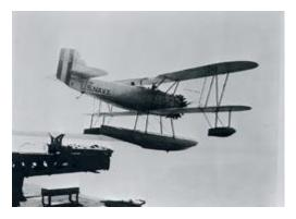
Using the new Pratt & Whitney 425-hp, air-cooled engine, the Corsair's tactical flexibility rapidly earned it the reputation as a jack-of-all-trades. They could be flown on wheels from an aircraft carrier as a defensive fighter, catapulted as an amphibian from battleships and cruisers, and land on carriers for re-servicing. For strictly water use, the amphibian landing wheels that Chance Vought designed could easily be removed and stored.
