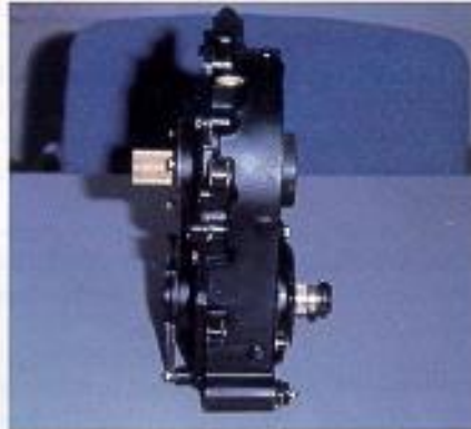
The fan gearbox is essentially maintenance free and requires only routine oil changes and inspection for metal in the oil. It is considered "on condition."
