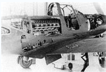
Bell P-39 Airacobra center fuselage detail with maintenance panels open.
