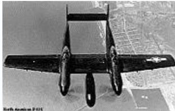
P-82C 44-65169 in black night fighter motif. Note the large bulge that carries the radar array, under the wing.
