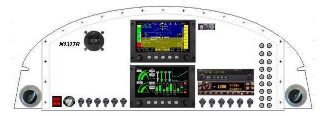
I think I can install Phase 1 myself. I will probably have a shop laser cut the panel. I may make a skeleton panel, and install the instruments in "thirds". That way, if I botch a panel, I don't lose the whole thing. It will better allow "phase changes" without leaving lots of big open holes in the panel, too.
