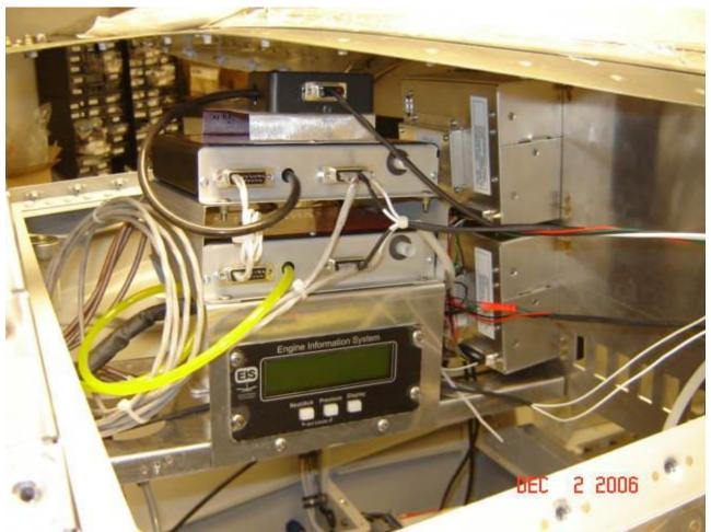
Note that in the pics above that I also mounted a little shelf above the top controller to mount the GRT MAP sensor. The two Plasma III controllers and the MAP sensor all have to share a MAP line from the engine. It was a convenient, albeit unsophisticated place to put the sensor.
