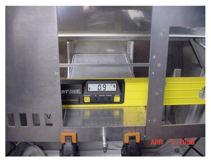
I set my digital level across the back of the tray, as close to the panel as possible. Reaching up under the panel while sitting in the pilots seat, I tweaked the center shelf to .9 and match drilled the right side. Then I double checked the level and drilled the left side. Then the center hole. So far, so good.
