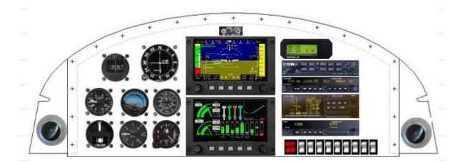
Off to the side could be a breaker or blade fuse panel. The appeal of breaker toggles is quite good. But lighted and lettered (engraved) rockers on the panel is what I would like best. Lighted rockers would have to be "full sized" in order to be engraved. The rockers above are the smaller "finger sized".
