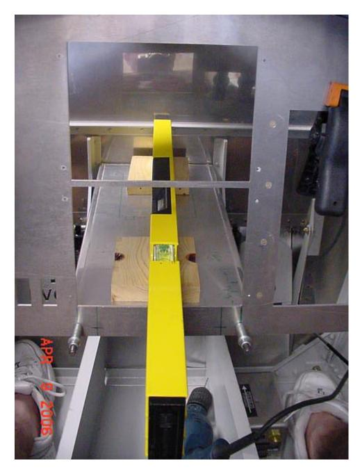
At this point, in order to level the shelf, I lined the top edge up with the top edge of the screen cutout. Interestingly, I had a scrap piece of would to set under the shelf across the master cylinder support brackets that perfectly leveled the shelf. Now I need to lower the shelf 1/2 inch on each end to keep it level and put the lower edge of the shelf at the lower edge of the instrument panel and out of the way of the 3.5 inch deep EFIS screens sticking down from the canted panel.
