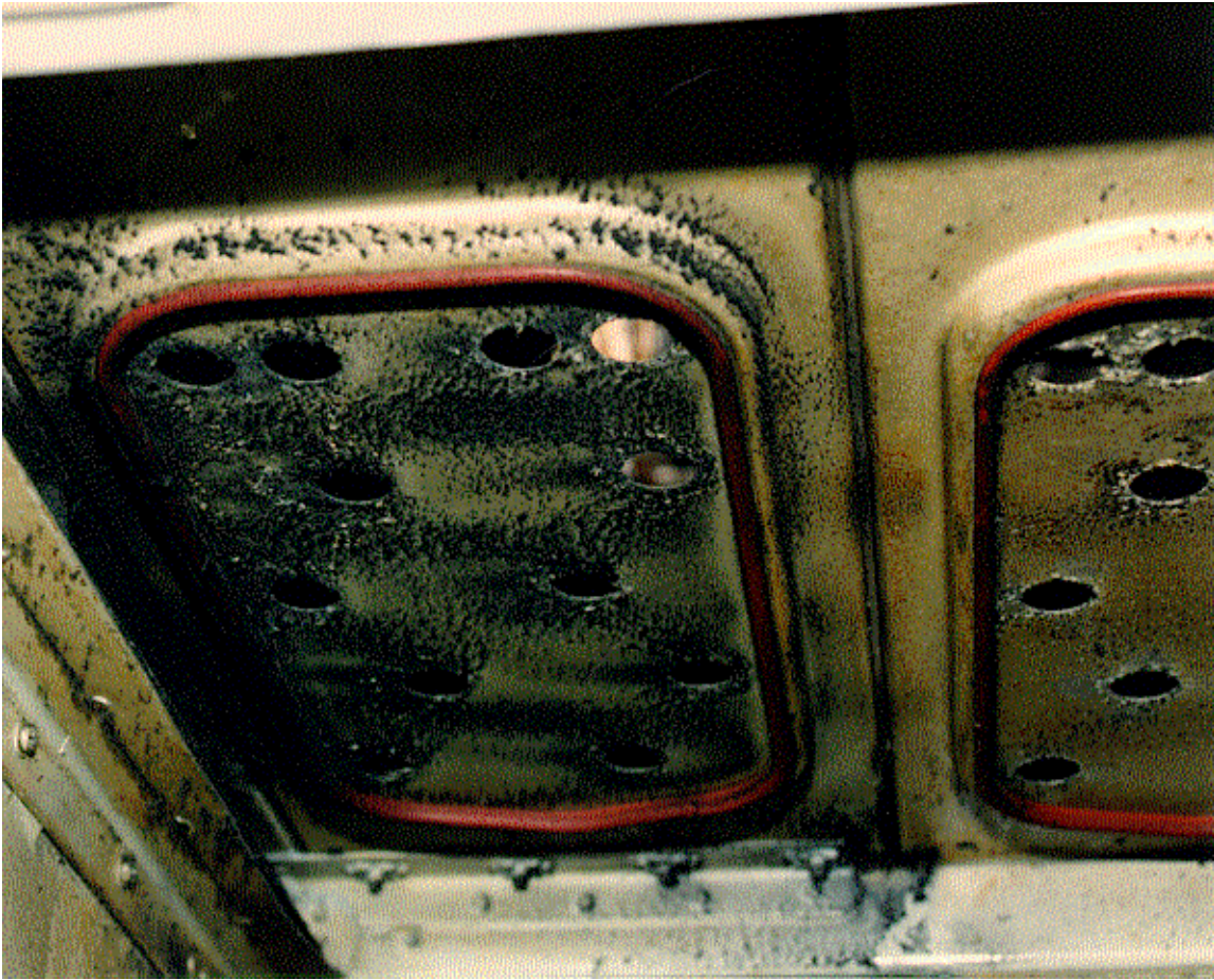
FIGURE 3-6. LINT ACCUMULATION ON AVIONICS RACK COOLING AIR MANIFOLD
