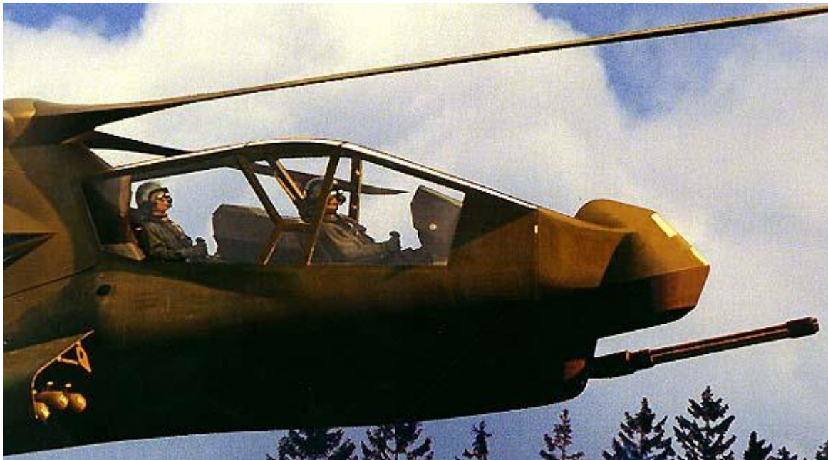
The Comanche is equipped with a stowable three-barrel 20mm gatling gun from General Electric.
