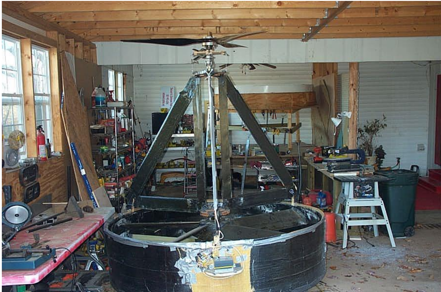
Radio controlled, US Patent Pending HoverCopter Prototype made from carbon fiber, foam and epoxy. Weighs about 200 lbs.
