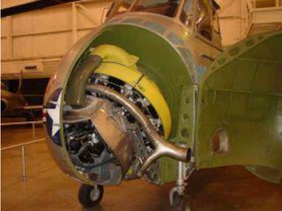
Pratt & Whitney R-1340 radial engine mounted in H-19 Chickasaw helicopter
