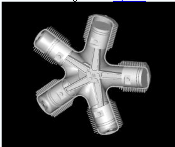
Radial engine with cut-away housing.
