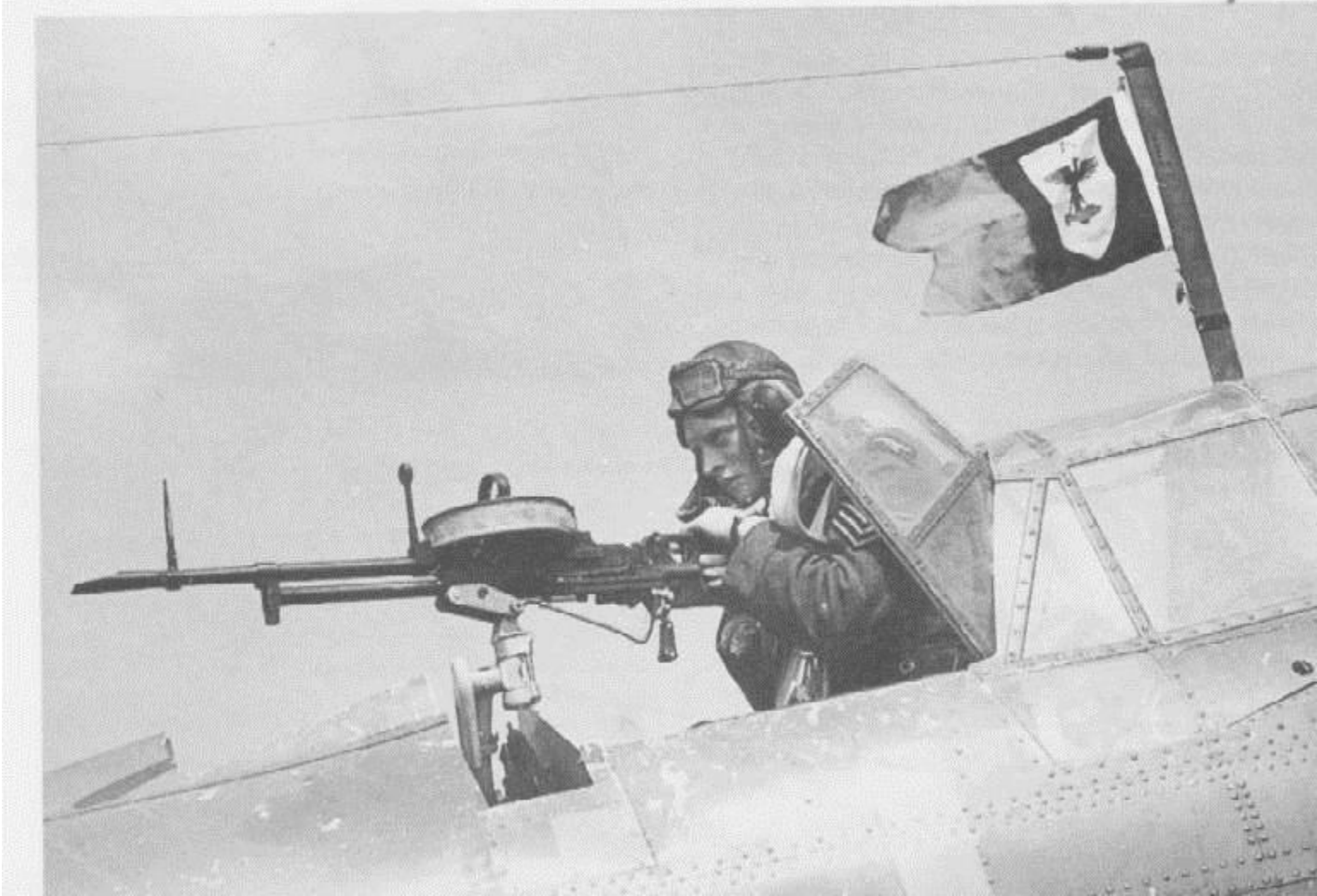
Fairey Battle observer using a 2 in ring and bead sight on a Vickers K gun
