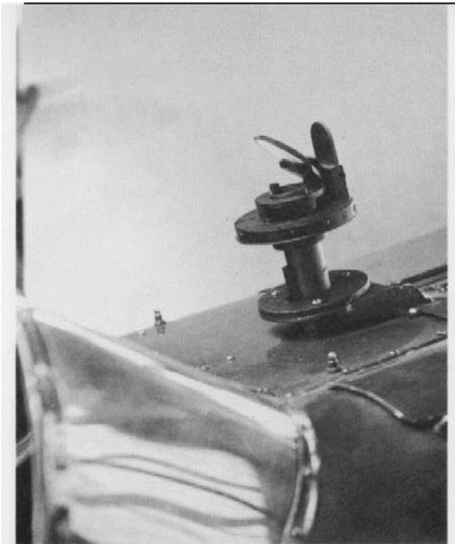
The Ogee ENI reflector sight of 1931, tested on a Douglas O-25A at Wright Field (Ross Whistler)
