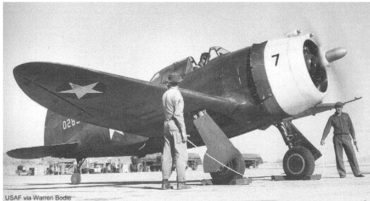
A P-43A in USAAF Training Command service, circa 1942. Note the revised tail wheel assembly.
