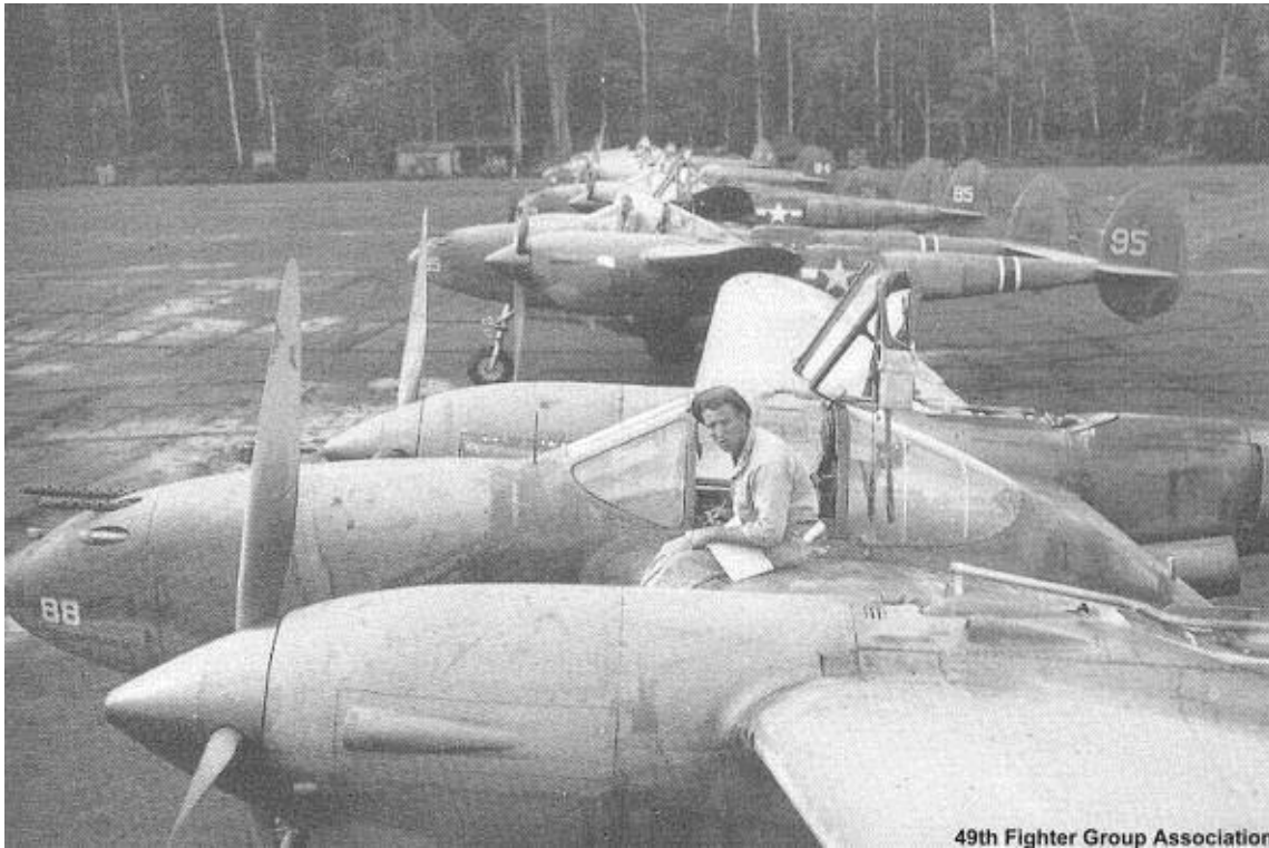
The war weary P-38s of the 9th FS sit lined up. Note the odd looking pipe installed on the turbocharger on the fighter in the foreground. This field modification provided additional "ram air".
