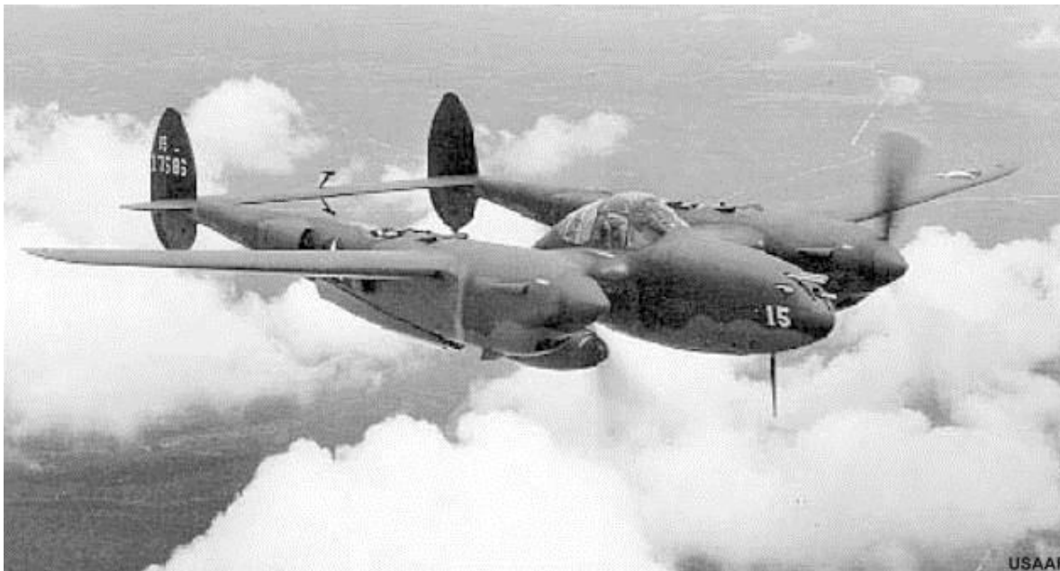
General Kenney certainly preferred the P-38 over the P-47 because of the Lightning's remarkable combat radius. This is a P-38F-1-LO, a later sub-model of the P-38F type was used by the 5th Air Force.
