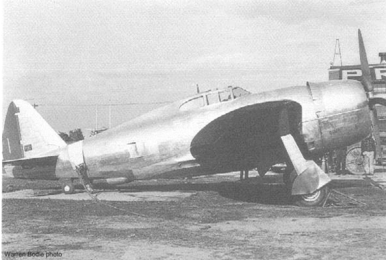
Tied down and chocked, the prototype XP-47B is readied for a maximum power run-up the day before its first flight.
