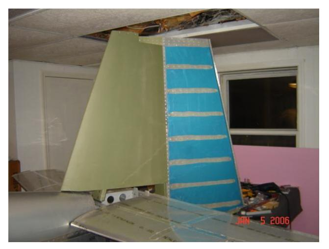
The manual calls for "30 degrees R/L" Now I'm stupid, and I don't know if that means 15 each way or 30 each way. I looked in chapter one and it says the same thing. Since the other control surfaces move 25+ degrees for the most part, I'll ASSume that I am supposed to be able to crank that rudder 30 each way.
