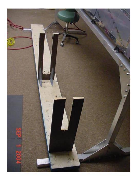
I mounted the boards on my handy beam that I used earlier in the construction of the HS and VF. I put the boards PERFECTLY (hah!) along one edge and marked on the beam 41 inches on center. I used a speed square to make sure the boards stayed square when screwing down the boards with shelf angle brackets. I then verified that I had 41 inches along both sides of the fixture between the boards.
