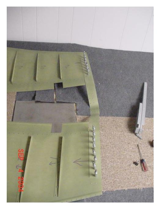
Before re-clekoing the parts, you have to re-bend the corners of the counterbalance. Then cleko these REAL tight. I riveted this area first, from the leading edge back. Then I put the assembly in the wood fixture and riveted along the spar. Then back on the bench, I inserted the R22 skirts and riveted along that side.
