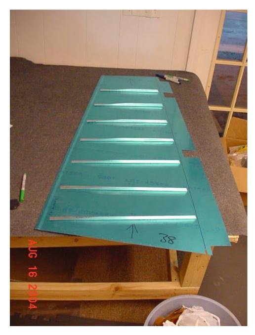
Notice in the pic above how the taper is to the doubler (aft) side of the skin. Also notice that the "open" side of the stiffener faces the same direction as the arrow. Just for good measure, I put numbers and arrows on the stiffeners and near the line of holes they will be attached to. It's VERY easy to get confused.
