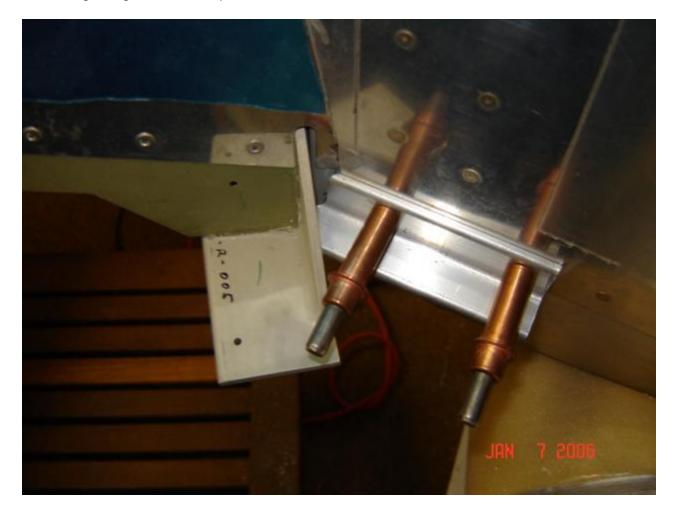
The stop isn't particularly aerodynamic, so next thing is to shape it up to reduce the weight and drag.
