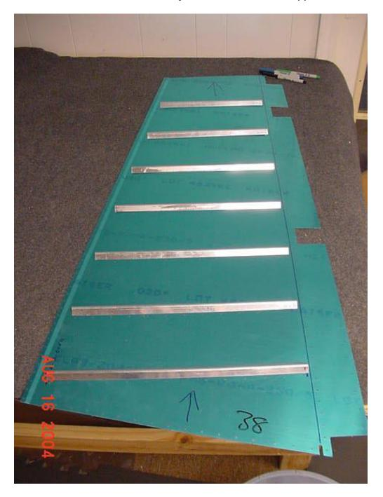
The bold line on the right is where the spar sits. The arrow at the bottom shows where the "open" side of the stiffeners will sit. I marked 1/4 inch on either side of the outer holes and cut all the pieces to length. The layout shows the approximate position of the stiffeners. I don't know what the 38 is at the bottom. Something the Czechs wrote on there.
