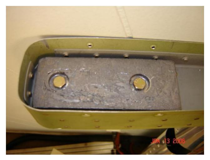
The Van's kit was pricey at \$6 each block plus shipping LEAD, but it was worth the hassle reduction. I attached the CW block with the rudder off the ship. Time to pin it back in, and run the rudder cables to the rudder horn. Maybe attach the tailwheel and steering link after that.
