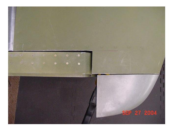
Scrap from my HS skins worked nicely for flanges on the rudder cap. These pieces are a little over 18 inches. Inside the counterbalance, the flanges of the skeleton are about 5/8 down from the top edge of the skin, so the flanges on my rudder cap have to be this long or a little less.
