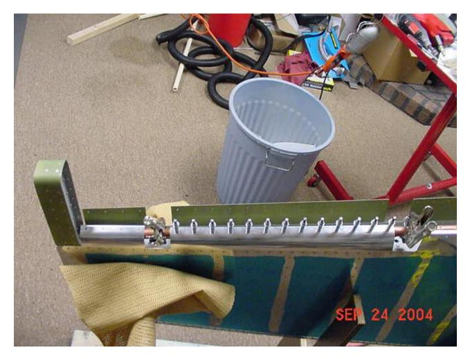
Once the skins are preliminarily rolled, I went back and coaxed the skins to nearly closed, i.e. the holes in the flanged skin are visible directly under the holes in the straight skin. Well, I couldn't quite get them to overlap nicely like I did the two elevators, but I got them pretty close.
