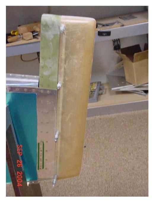
I ended up trimming down the top cap on the rudder about an inch shorter than the plans. I just didn't like how tall it was. It didn't look right. So my cap is under 4 inches at the leading edge and the trailing edge is about 3 inches.
