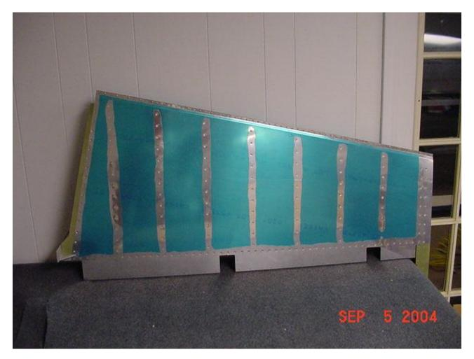
The rudder and VF have been sitting around for about a month, waiting for construction of their sibling control surfaces. I have rough cut the top part of the skin to allow for the counterbalance to swing though and have the VF primed. As far as metal work goes, all I needed to do on the rudder was roll the leading edges of the skin to curve at the hinges.
