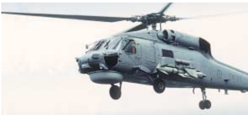
ASUW mission configuration includes Penguin missile, shown here in stowed position on left extended pylon
