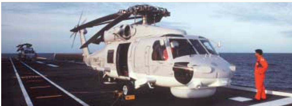
Main rotor blades fold to reduce aircraft footprint
