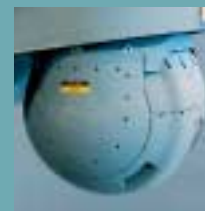
Forward Looking Infra-Red (FLIR) system
