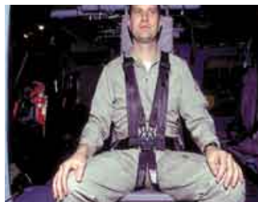
Troop seats with five-point harness provides maximum protection for cabin passengers
