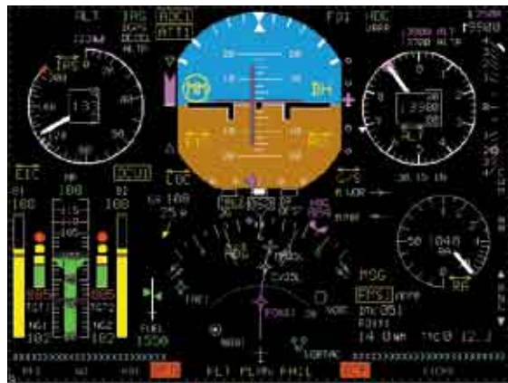
Digital multi-function display panels combine information from multiple analog displays, reducing cockpit clutter and aircrew workload
