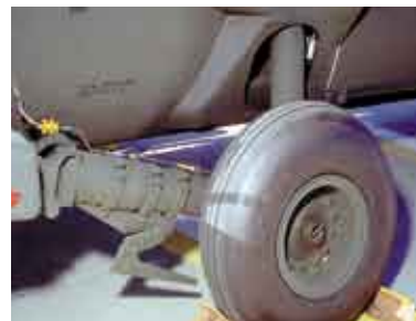
Landing gear absorb energy of up to 30 feet per second and provide wirestrike protection
