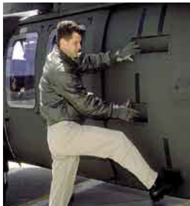
Retractable steps and recessed hand- and foot-holds allow easy access to entire aircraft
