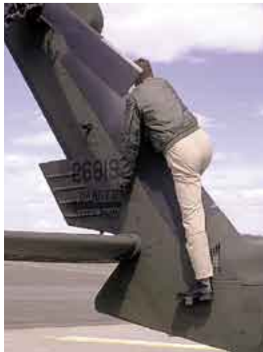
Retractable steps and recessed hand- and foot-holds allow easy access to entire aircraft
