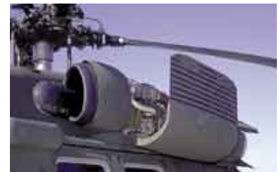
Engine cowlings which open to become stable work platforms and designated walk areas allow access and protect aircraft during maintenance
