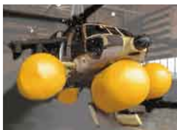
Emergency flotation system
