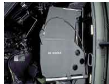
Swing-out armor side panels protect pilot and copilot from ballistic threats
