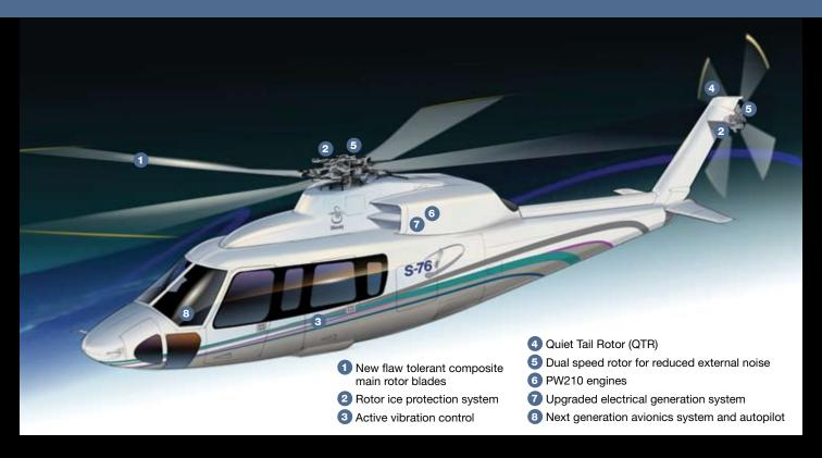
The Sikorsky S-76D helicopter has been developed in response to customer requirements, but in a way that will exceed operator expectations for safety, comfort and performance.
