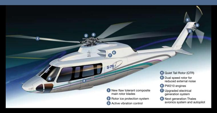
The Sikorsky S-76D helicopter has been developed in response to customer requirements in a way that will exceed operator expectations for performance, safety, and value.
