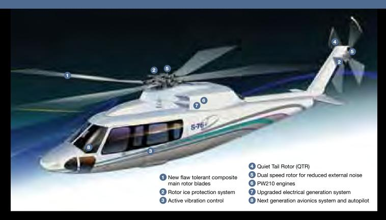
The Sikorsky S-76D helicopter has been devel- blades. New Pratt & Whitney Canada 210 engines oped in response to customer requirements, but in a way that will exceed operator expectations for performance, safety and value.
