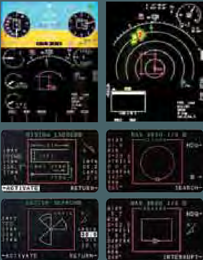
Superior SAR Displays: Pilots benefit from the S-92 Universal Flight Management System with Multi Mission Management System, which provides search patterns to multi-function displays.
