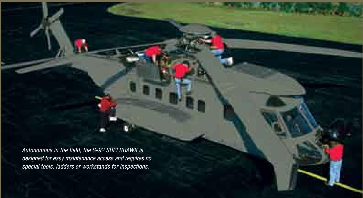
*Autonomous in the field, the S-92 SUPERHAWK is designed for easy maintenance access and requires no special tools, ladders or workstands for inspections.*
