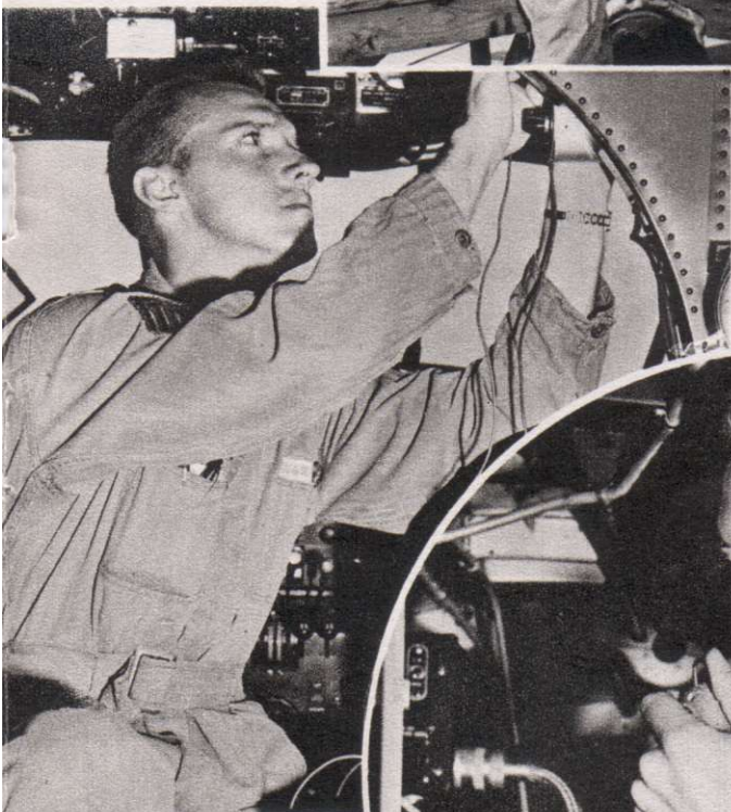
To insure the safety of the men who fly, ground crewmen check every working part of training planes. A technician using a test meter to check a plane's radio system.
