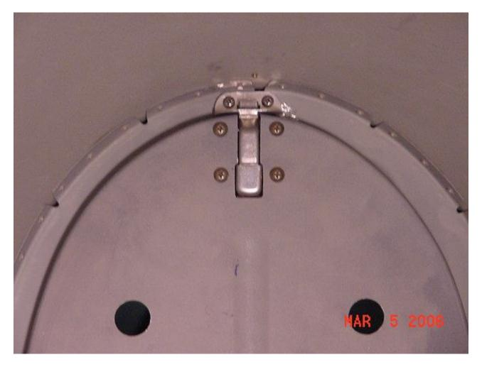
The hasp and Hartwell latch combination holds the close out door against the bulkhead quite nicely. The edges of the door are smoothed, but not completely finished. If I run across some edge trim, I may run a bead around the door so that it sits against the bulkhead without rubbing into it and getting sloppy over time.
