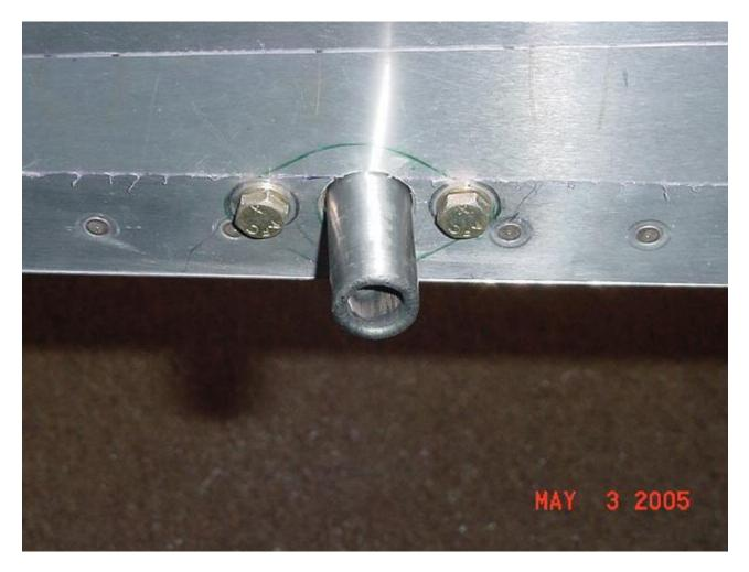
See what happens when I get bored! The tube sticks out about 1 3/8 or so on each side of the ship. The flap actuator arm goes on the end of the torque tube. It just barely fits on there. I still don't know which way it goes on the shaft. I'll hazard a guess:
