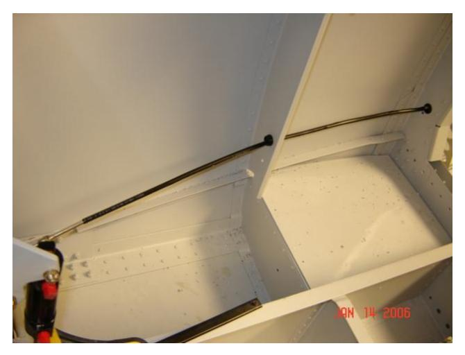
In addition to running Nylaflow over the steel cable to help it slide, I also bent the steel tab on the rudder pedal to help the swag have a straight run at it. I was sure to test the entire setup for full travel and clearance at the firewall footwell. So far no problems.
