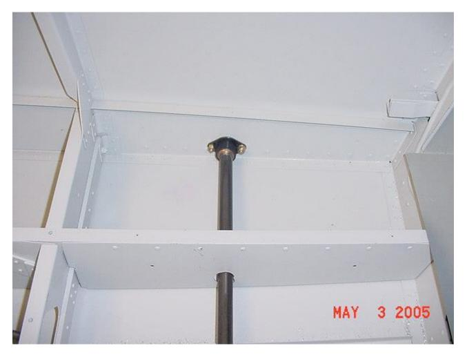
Don't be concerned about how much divergence there is at the sidewall. There is about 5 degrees of discrepancy between the torque tube and the side wall/bearing. The bearing is made to accommodate this difference. When you get the tube ready to insert through the bearing and sidewall, just gently tape the tube with a rubber mallet and the bearing center will shift to align with the tube. Neato, bandito!
