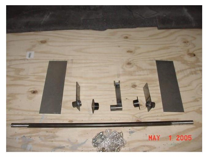
The torque tube has a specific orientation. There is reinforcing tubing welded to the inside. The end with two welds has a longer tube inserted in it. This will be the left end of the tube. That is of course to reinforce the motor attach bracket area. The motor attaches to the left side of the #7 bulkhead.
