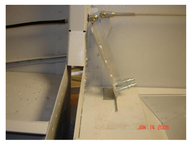
From the beginning I new that I could not just run these steel cables and expect the plastic grommets to hold up. Therefore, I also bought some NYLAFLOW 1/4 inch tubing. I slit the tubing and more or less spiral wrapped the forward cable completely. That material glides on the plastic grommets beautifully.
