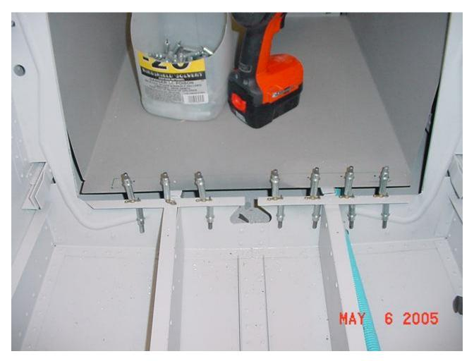
Placing the seat back hinge was pretty straight forward. I just put the corrugated seat back fully back in place and marked were the hinge goes on the floor. I did have to reverse the hinge that screws to
