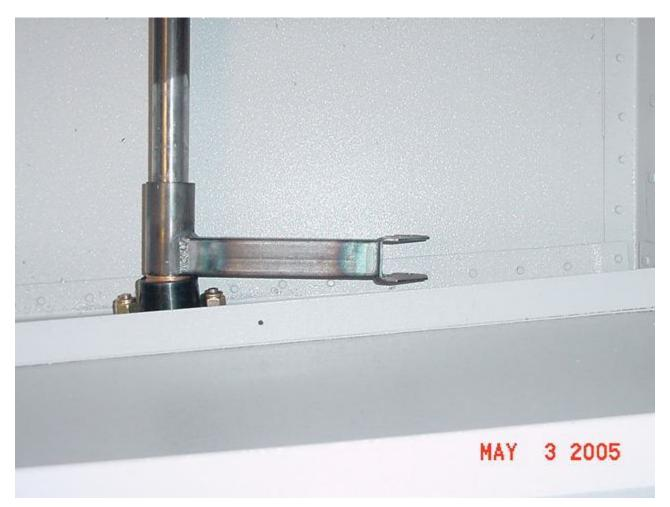
The flap motor armature barely clears the rib without hardware. With hardware, it's going to take some trimming. I hope the motor arm attaches with a clevis pin instead of a bolt, otherwise it's going to take some major cutting!
