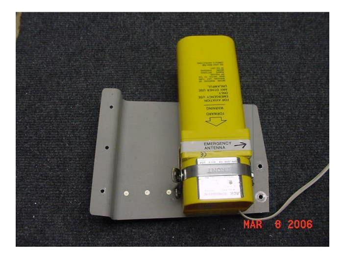
With the ELT and it's tray set back, I can now remake the baggage floor and the "hat rack" "battery cover" and gain 4 inches of storage space behind the back seat!
