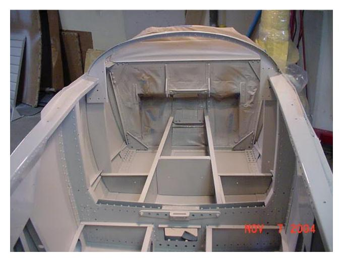
I finally got around to painting the interior of the fuselage. It took longer than I thought. I used a touch up gun through the first top coat. I was trying for a textured effect, but didn't really like the results. The color looks great and the material is tough as nails, but it certainly could have turned out better.
