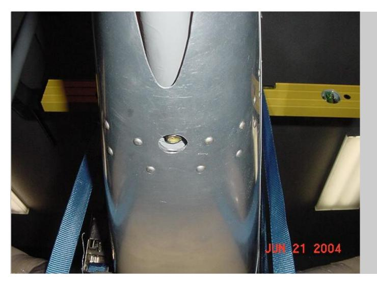
You get to drill a 3/4 inch hole in the bottom of the empennage. You can see it in the pic with the tailspring bolted temporarily in place. It turned out very nicely (so far). There is no slop with the bolt in place, and the hole through the spring and the bottom of the airframe are very centered and vertical.
