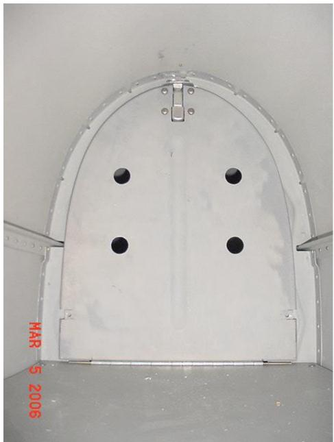
I ended up using a Hartwell latch I bought from Wicks on close out for about \$2. I had already notched out the top of the close out door, so I went the rest of the way and installed the rather large Hartwell. Then I attached it to the door with #6 ss hardware.
