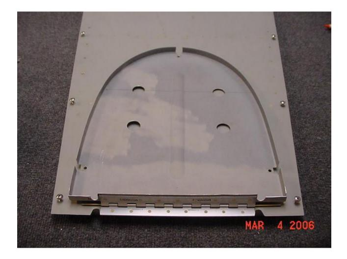
Along the side of the aft baggage floor, I only used 4 screws each. Instead of trying to rivet in nutplates, I chose to use tinnerman nuts that clip onto the longeron and then use #8 stainless sheet metal screws to hold the floor down. The KISS rule applies here.
