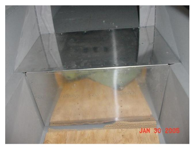
Now that I've remade the hat rack to compensate for moving the baggage floor pan, I decided to remake the baggage floor pan and extend it aft about 4 inches. Since my EVO battery was moved up front, there is wasted space under the hat rack and behind the floor. I thought I should take advantage of it, even though with the EVO CG a little farther aft than the standard F1, I may not be able to use the extra space as I would like. But anyway, now to remake BOTH parts.
