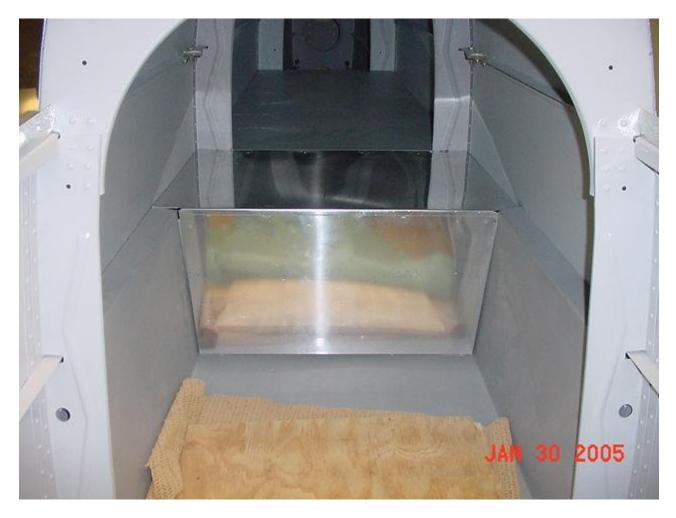
I made the whole part out of .025 that I bought from Wicks (about the cheapest I've found). The piece is about 1/8 wider at the top to allow for taper of the ship, and I extended the top to about 11 1/8 inches. Trimmed to fit, match drilled for the #10 screws, countersunk the brace of the rear floor, dimpled the hat rack, screwed it down with 10x6 cs ss screws ET VOILA, FINI! Easy when you have a little rolling/bending/shear machine.
