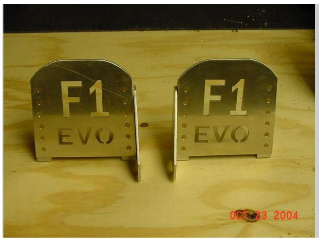
I had measured and drilled these parts a while back. Since there is so much symmetry in these parts, I was able to match drill each flat pair. I.E., I drilled the pedal plates and the actuator plates that rivet to the side of the angle pieces together.
