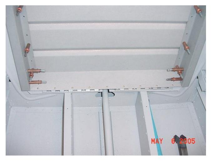
This worked pretty well. The seat back sits against the bulkhead quite nicely. Later on, I'm going to cut the lip of the flange on both the bulkhead (as little as possible) and the seat back (as much as needed) to improve how it sits. Making it sit more "flush" will actually set the seat back at a bit more of an angle. It will also allow some clearance to attach some rubber channel on the lip of the seat back to cushion it on the bulkhead.
