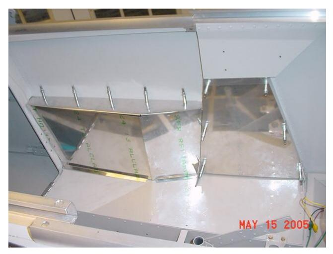
Next I have to decide how to assemble the arm rest and it's side panel. The trapezoid panel is easy. I'll use #6 or #8 screws and nutplates there. The arm rests are another story. Randy Pflanzer riveted his arm rest top to the longeron, then made the side panel removable with screws along the top and bottom of the side panel.
