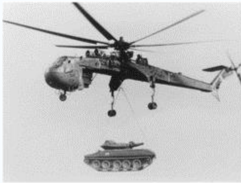
CH-54 Tarhe carrying an M551 Sheridan tank on a sling mount in Vietnam.
