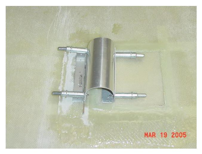
What I found was that the best operation seemed to be when the apex of the curve in the rolled body of the hinge sat directly above the lip of the opening. My rolled piece is nearly round, so this was kind of a no-brainer. I've seen hinges like this that were no where near round and so the apex above the lip would not work that way.
