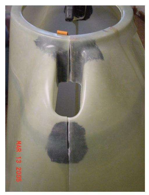
You can see the discrepancy in the angle of the short tape on the side of the spinner opening/air inlet. The angle should be the same as along the long side. Oh well, the beauty of fiberglass is that it's repairable. I've repaired enough small fiberglass parts in my day (wheel pants and other cowls) that I'm not distressed. Just bummed that I'm starting out this way. Drat.
