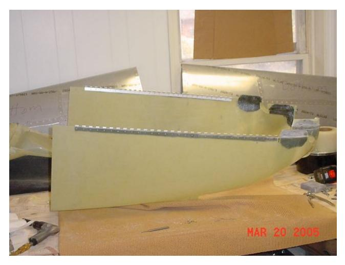
After completing the 4 hinges, I went back and cleaned the area around the hinge eyes and rivets. Then I ran the pins through. No problem there, just a little tighter than before. I figured I had better go ahead and pin the halves together while the JB sets up, just to ensure the best alignment.
