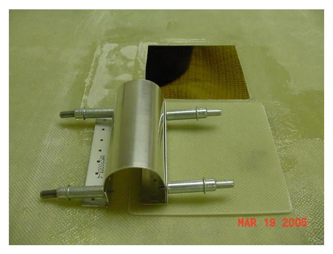
The plans recommend that you use doublers to level the hinges. I won't need to do that, because the layers of fiberglass I've put on to reinforce the hinge area also serve to bring the level of the hinge down to the level of the stepped lip in the cowl opening. Actually, with this method of oil door hinging, you don't need the thickness to level the door anyway. The rolled body of the hinge is very adjustable, and will allow you to level the door very easily.
