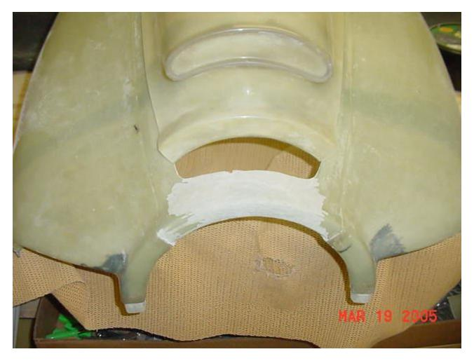
After a few hors of sanding and grinding, I finally got the POS air scoop to fit on the lower cowl. It seats rather nicely now, thanks to lots of stupid cheap labor... me. Once the scoop was fitted, I went ahead and cut the mount open. That alone took about an hour to cut and shape and smooth.
