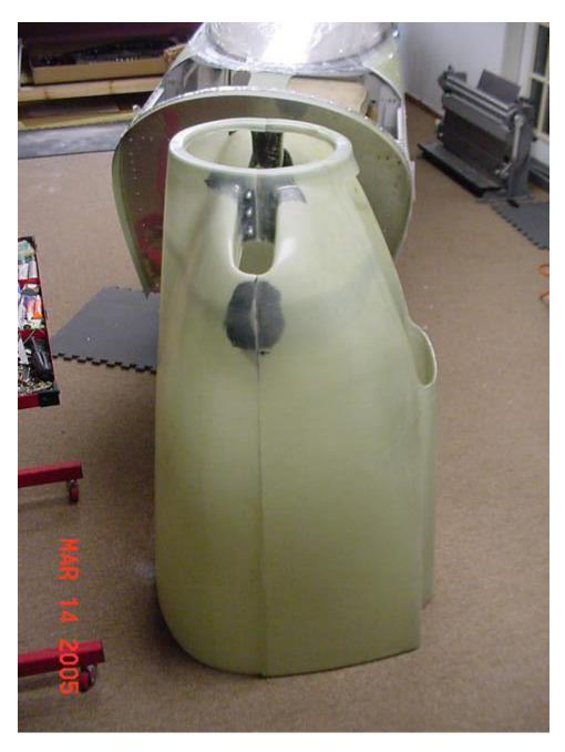
With 6 clekos in the cowl, it really wanted to sit together nicely. The horizontal cuts on the sides of the cowls are pretty close. It's not flush sanded yet, but it's close. I have to verify the size and shape first, then I'll tweak the alignment top to bottom. So far, so good.
