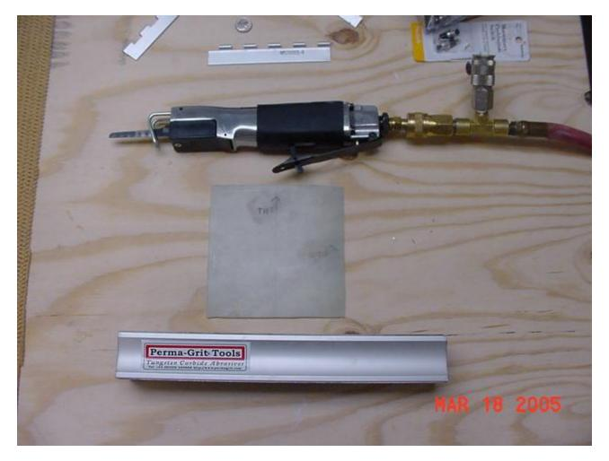
The oil door comes scribed, so I used my air saw and cut it right to the line. Then again, I used my Permagrit block to square it up and smooth it off. The door sits in the recess of the cowl rather nicely without any cleanup of the cowl. The recess is just right. You can adjust the door on the engine side if you want it to sit better..
