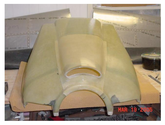
Then I cut the big air hole (where the air scoop attaches) in the lower cowl per plans. 7/8 on the sides, and 1.5 inches at the front. The rear is a guess. I left it alone. It isn't hurting anything. You are supposed to radius the corners to 1 inch. I looked at the pic in the plans and guessed. Looks good to me!
