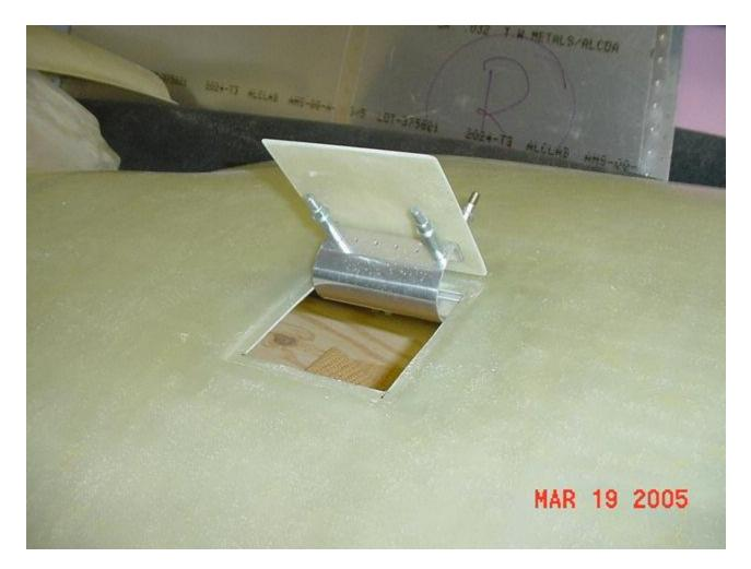
The door actually opens more than shown in the pic above. The clekos are interfering with the full travel of the hinge.
