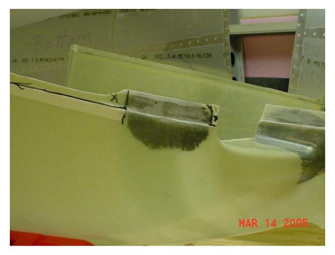
We finally got our communications straight and Mark confirmed a couple things not laid out early in the plans. The area of carbon fiber on the lower cowl near the front is indeed left for an alignment and support tab. It should be about 4 inches wide by about 1 inch tall. All the tabs and overlaps on the cowl halves seem to be about 1 inch wide.
