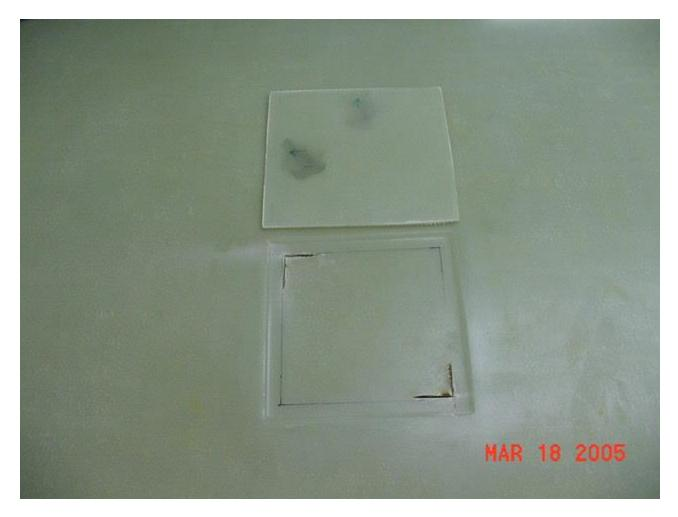
The plans suggest 5/16 to 3/8 inch border around the cut out for the oil dipstick door. I did not make provision for cam locks in the corners. I measured a liberal 3/8 around the inside of the oil door recess on the top cowl. Then I took my dremel and made corner cuts that were big enough to be able to follow through with my air saw. I used my Permagrit block and smoothed the inside edges.
