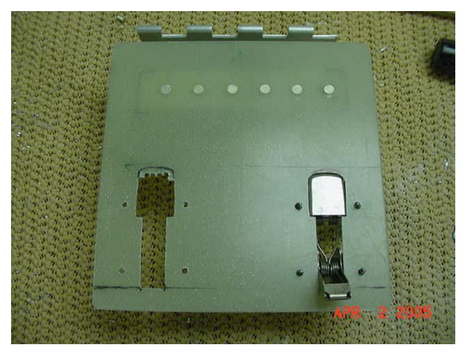
The rivet holes in the latch will take a #3 countersunk rivet, probably a -5. I'll cs the oil door and squeeze the rivets in each corner of the door. And that will complete the latches and the oil door. Then I just have to insert the hinge pin and fasten it down. Very nice little project!
