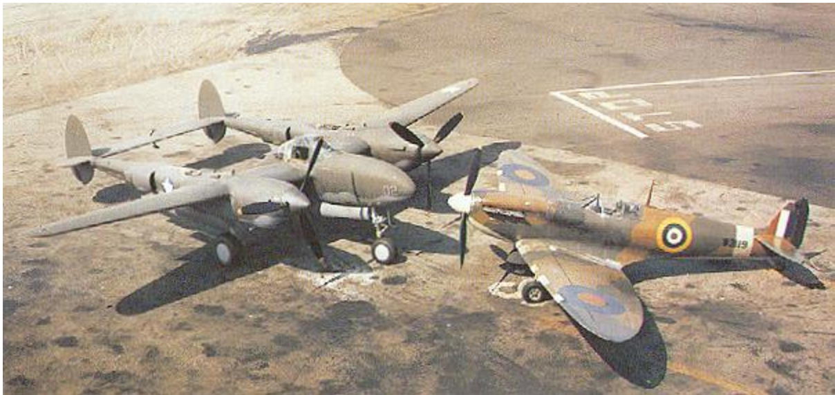
Pictured is a P-38F-5-LO and a Spitfire Mk.Va on the Lockheed ramp. While the Lightning is larger, with its twin booms, the distinctive wing shape of the Spitfire is a dead giveaway as well. LAC via Warren Bodie
