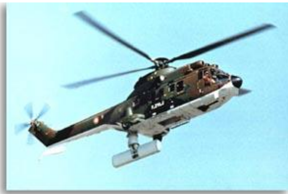
BATTLEFIELD SURVEILLANCE Capable of processing 4000 targets simultaneously, the "HORIZON "system is designed primarily for observing ground movements and for target designation up to 200 km.
