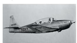
low-wing monoplane with an aluminum fuselage and tandem cockpits with dual controls. Although it was flight tested successfully, it did not win the competition.
