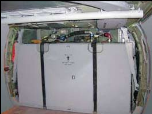
Auxiliary single fuel tank installation
