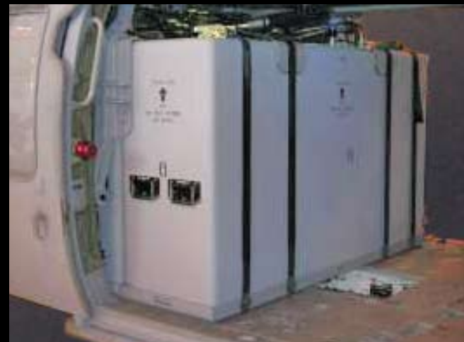
Auxiliary dual fuel tank installation
