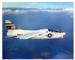
was bailed to LTV by the Navy. In a whirlwind design and manufacturing effort, the V-519 was born. Built on temporary tooling, and making maximum use of A-7E design knowledge and existing parts, the "White Whale", as it affectionately became known, took to the air in August 1972. Later it was redesignated as the YA-7H and ultimately became the YA-7E.
