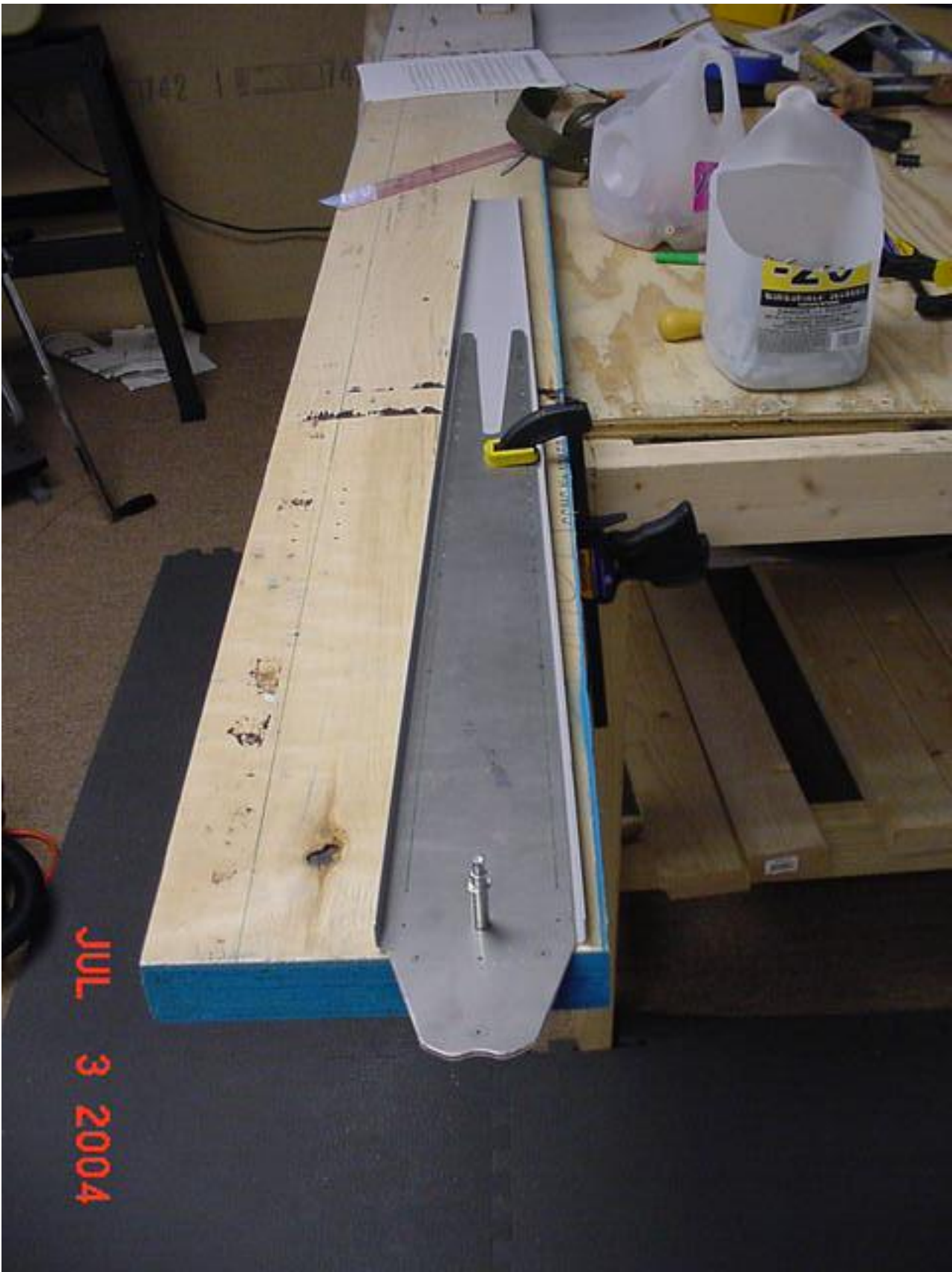
Once you have the two parts drilled @ 40 and then clekoed together, you start adding the pivot brackets that the rudder will swing on. The process is the same as with the HS, except that 2 of the 3
