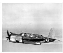
A mid-wing monoplane, the three-place Sea Wolf was a large machine powered with the big 1800-hp P&W R-2800-6 engine,a wing span of 56
