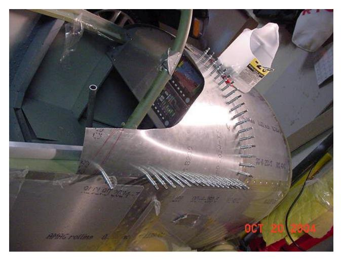
After some time, I got the left windshield skin ready to drill. I tried my shrinker to try and get this one to lay in the angle part of the fuselage better. It was to no avail. I don't have a vice anchored down, nor a handle sturdy enough to operate the shrinker. In the end, I used a hand file and my 3in1 bending break to cut the wonky angle at the bottom of the skin.
