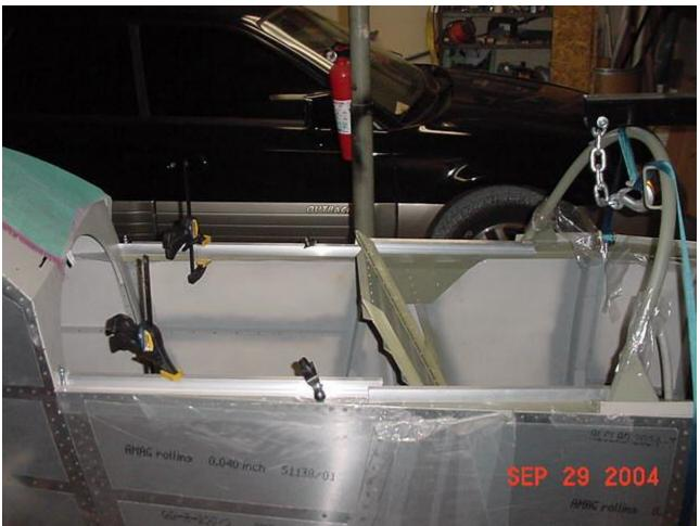
With the removable notch made in the canopy track, I positioned the rear pieces against the #7 bulkhead and trimmed the aft end flush to the bulkhead so the tracks would be identical and to sit in position.
