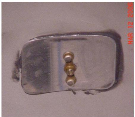
I typically don't have anyone to assist me while working on my F1. Putting fasteners inside the ship under the canopy track would normally be a two person job. I wanted the track to be relatively easy to remove, so I decided to put nutplates in now, rather than nylock nuts, back in the empennage under the canopy track. I also wanted to install a fasteners by myself without resorting to bucking anything on the skin if at all possible.
