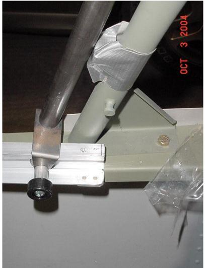
I used 2 NAS rivets in the forward track brackets to tack them to the tracks. First, I Epoxied all four angle brackets in place. I was unable to get a squeezer on rivets in the aft track, so I'm just leaving them epoxied. If they come loose in service, I may have to grind off the center spline in the middle of
