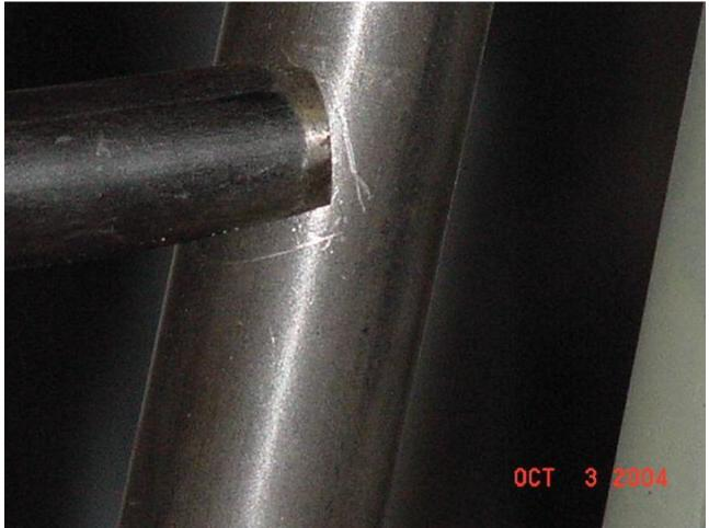
My FB was marked from the factory with a deep scratch precisely where the Horizontal Canopy Bar goes (HB). The horizontal bar sits with the large round weldment parallel to the welded closure pin on the Windshield Bow. These parts need to line up to latch the mechanism later on.
