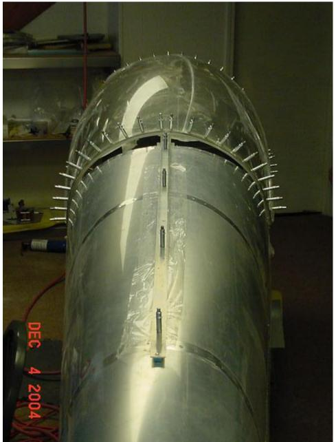
While working on the slider, I had to attach the frame to the canopy track. I installed the plastic "glide" block that bolts to the frame and slides along the track. During the early phase of slider construction, I just had the track duct taped to the turtle deck. After a while, as the slider became more complete, I contemplated attaching the track to the ship.
