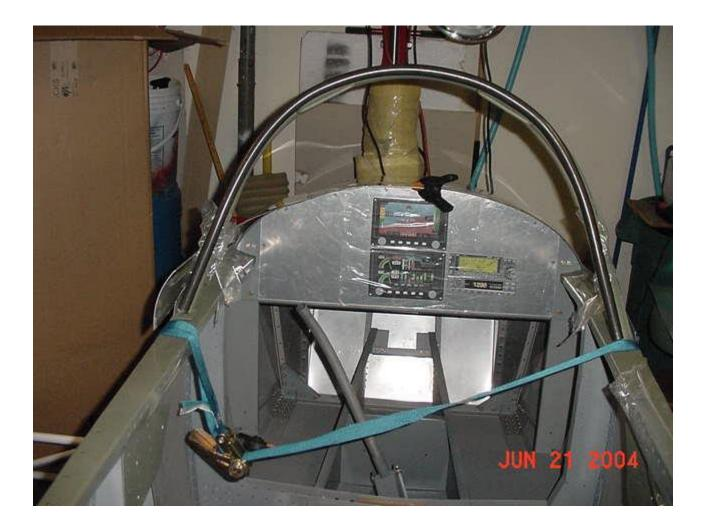
I set the front canopy bow (FB) in place and checked how far over the top of the windshield bow (WB) the FB extended. My factory length FB bent to match the WB was about 1 inch over the top of the WB sitting on the canopy rail.
