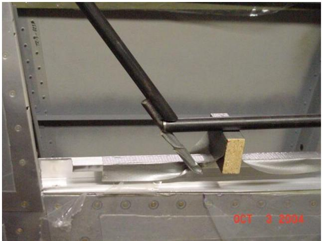
The RB slider sits on the center track and the way the factory has prepped the parts, the HB kind of locks against the anchor pin and under the very end of the RB tube. Again, with Randy's measurements and the factory cuts, this all fits together beautifully. By this I mean if you hold the frame together this way, you also get that 1/8 inch clearance between the extended line from the top of the center track and the top of the rear bow. Neato, bandito!
