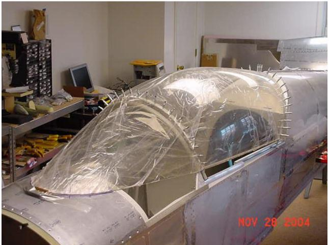
The canopy center track had to be moved forward about 1/8 inch to raise the rear bow a bit. I think the weight of the Plexiglass was enough to sink the frame on the unsecured track (just duct taped at the aft end). Not a big deal, but the ss latch pins at the back were dragging on the side tracks. Not good. I'll probably have to adjust this again later, it still isn't fixed in place, and it's a good thing.
