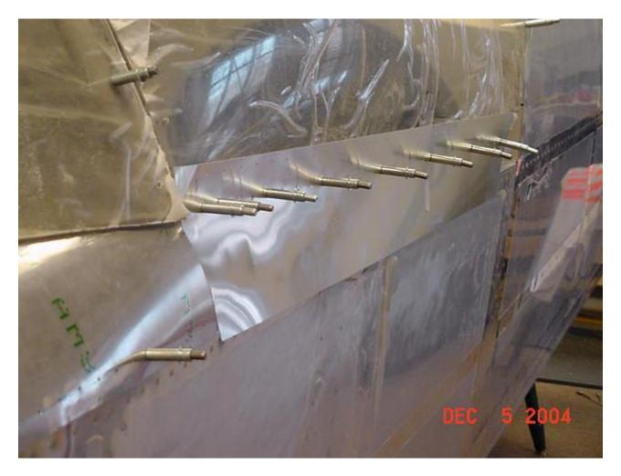
I've decided to remake at least one of the skirts. The 2 elongated rivet holes and the ripples in the lower edge where I flanged it are going to look like crap. I don't think the rivet head would even cover the holes, and I can see the rivet spinning and making a black dust mess down the road. I'll keep the skirt, just in case. The roll/bend in it turned out very nicely, and the botched skirt will at least make a good template.
