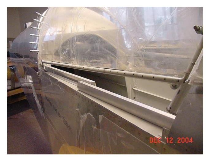
My apologies for the above pic. There is a black line drawn where the top of the skirt and retainer sit. There is a red line drawn below that to correspond with the depth of the retainer piece (C059). That makes it 3/4 inch below the top edge of the skirt/retainer assembly. That's how I determined that I have to cut another 1/4 inch off the plexi. And I'm sure the left side is the same way.
