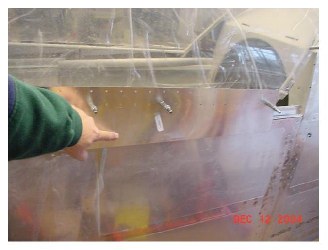
You can see in the pic above where I was tapping, and how far aft the contact point was after making the "S" roll in the leading edge of the skirt. Once I drill all the holes, I'll cleko every hole and check this relationship again.
