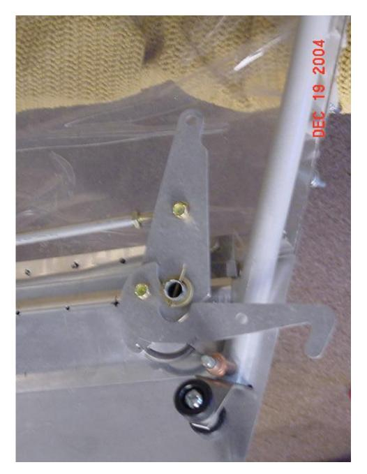
What the heck... I grabbed up the latch connecting rods and some AN3 bolts, nylock nuts and washers and trial fit the whole thing together on both sides. FUN! I like bolting stuff together. I'll let you in on a secret. I never wanted to BUILD a plane, I really just wanted to ASSEMBLE one. There's a difference. Today there was a lot of assembly, and it was a nice break from the drudgery of fitting the skirts. That was depressing me. Anyway, I'm re-energized and ready to rock.
