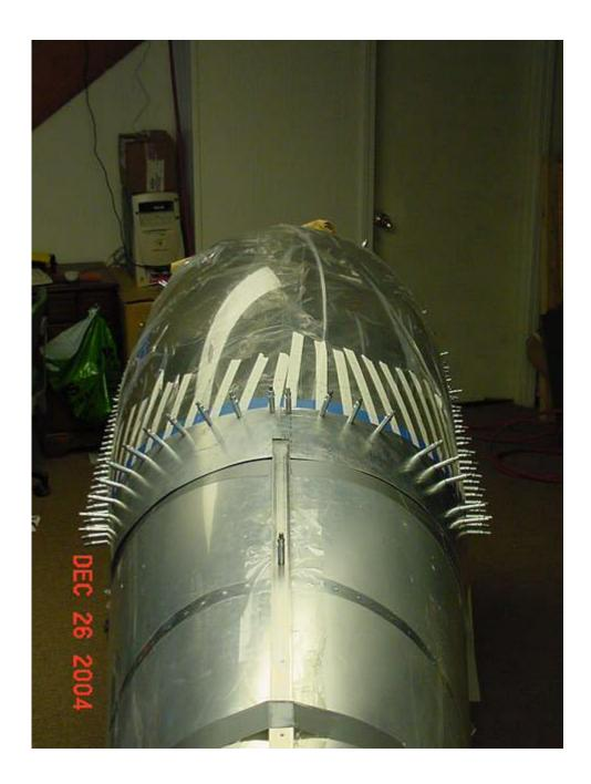
I will also have to remake the fairing for the center track. Getting that piece to bend at the proper angle has turned out to be quite the bitch. The problem is that I can't make two bends on a piece of .032 that taper to a fine point on my break. I think I'm going to end up using a flanger and make it by hand.
