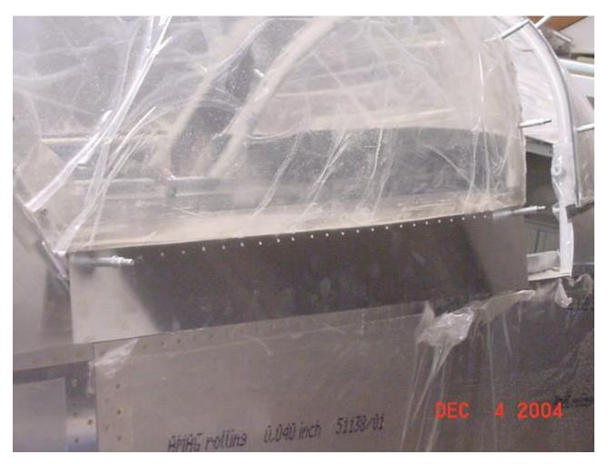
A couple warnings: I got disoriented and drilled the second set of side skirts backwards. I drilled the C059 from the front, not the back. Fortunately, I was able to reverse the C059 and the holes were close enough to still work. Luckily, none of the holes in the C059 retainer will show anyway.
