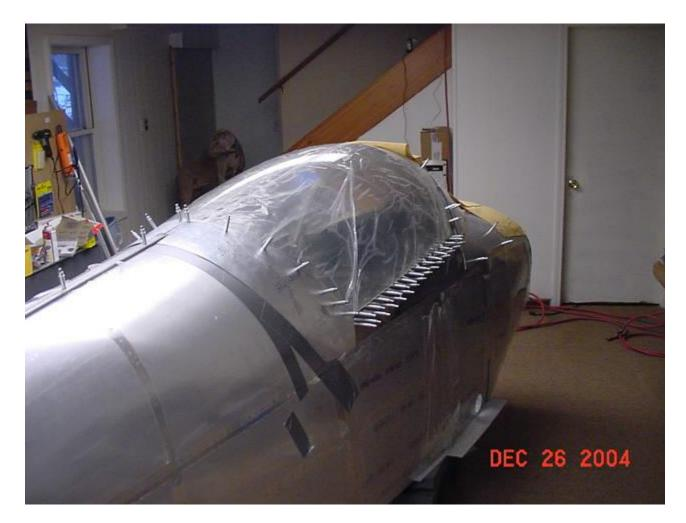
The skirts still required some rolling to improve the relationships at the top and bottom. The part overlapped at the top, and now have a butt joint. There's going to be a butt joint at the bottom, too, where the rear mates to the side skirt. I will make a doubler for each side and rivet them in place.
