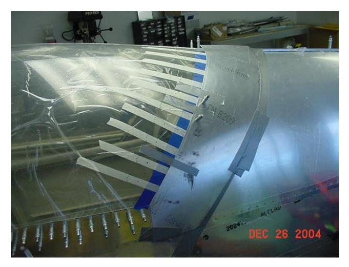
Now that the rear skirts are clekoed in place, it's time to do some trimming. First off, I got on a chair and went to the top of the ship and marked the "slot" where the center track goes between the skirts. I marked this area and cut out both sides with the dremel. I also marked the bottom and "mating" side edges to correspond with the side skirts and cut those on my 3in1.
