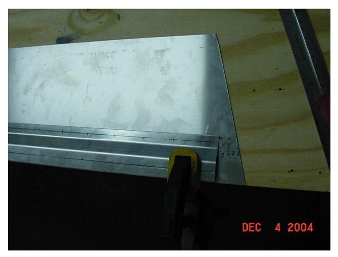
Back at the bench, I centered up the pieces and got them looking good. Contrary to the plans, there is no offset in the plastic piece, it is now made as wide as the retainer "slot" which is 3/4 inch. I drew a center line at 3/8 (I figured that out all on my own!) on the c59. I also drew a center line along the other rivet line where the sandwich of the C059 and the skirt are riveted to the horizontal on the slider frame.
