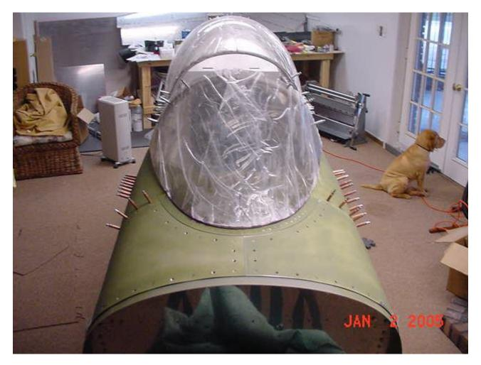
I put the SSW back on the bow for funsies. I marked the lower edge of the glass on the WS and the boot cowl arc. Time for a little painting. Flat black on the glare shield underneath, and on top under the glass. Then it will be time to get those Windshield Skins installed.
