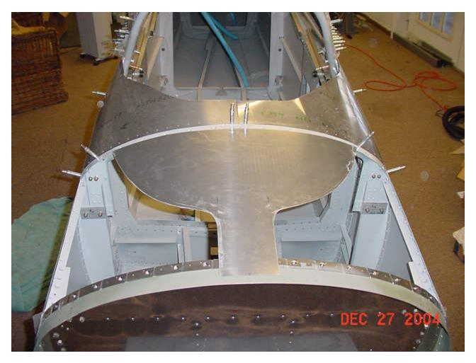
I wanted to make sure the doubler didn't interfere with the flange that the arc screwed to, so I got a marker underneath the arc and traced the flange at the aft end. I took the arc and the doubler to my bench and put them face up, flush at the aft end and centered. I used the screw holes in the arc as a template to orient the first round of rivet holes in the doubler. I went ahead and drilled the "screw holes" with a #40 bit.
