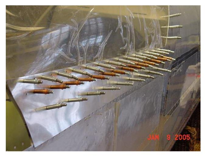
Once the steel holes were drilled up, all the side skirt parts came off, I sat in front of the TV making blisters on my fingers with a deburring drill bit. The side skirt assemblies are ready to sand, prime and dimple.
