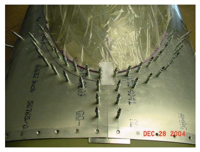
More thoughts on the move to change the boot cowl arc under the SSW: There are K1100 nutplates spaced two inches apart. If I drill them out, the area where the nutplates used to be is worthless for riveting. That means I might be able to get two rivets in between where the screw holes used to be. Is that going to be as strong as the screws? I don't think so. And this is a structural assembly.
