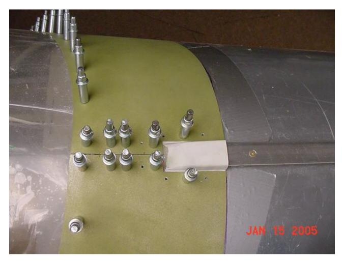
One thing I did on the track fairing was to trim back the aft edge. I cut the flange back at an angle, pretty close to the aft rivet holes. I also thinned the fiberglass to paper thin at the aft end. In the pic above, the last two clekos are actually touching the turtleneck. I probably should have skipped the aft two holes. I'll use NAS rivets here and mash them down to next to nothing. All the other rivets should clear just fine.
