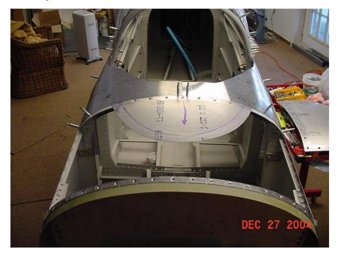
For now, I have cut the arc and separated the boot cowl into 3 pieces: the arc and the L and R halves. After cutting them with the dremel, I immediately took all the parts over to the scotchbrite wheel on my grinder and smoothed all the edges. After I screwed that parts all back down, I was amazed that they went back together so well. Virtually all the gap that was visible between the pieces was the width of the dremel wheel. SWEET! Still perhaps too wide for most people's tastes.
