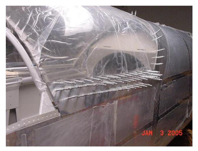
The WB is off the ship, and I ground off the rear ends of the base to allow more clearance at the canopy tracks. I re-primed that area and I'm going to put a second coat of PPG gray over everything.
