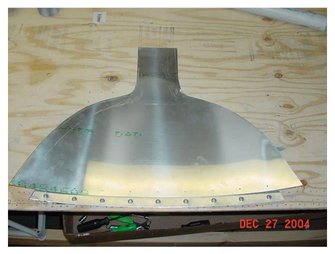
Over at the ship, I screwed down the arc, and clekoed the doubler underneath (although the "tongue" just lapped over the firewall flange). I went ahead and partially screwed down the boot cowl halves. AMAZING! IT WORKS! The parts all pull right back down and actually look pretty good! The gap at the arc cut looks about the same. So that's good to go!
