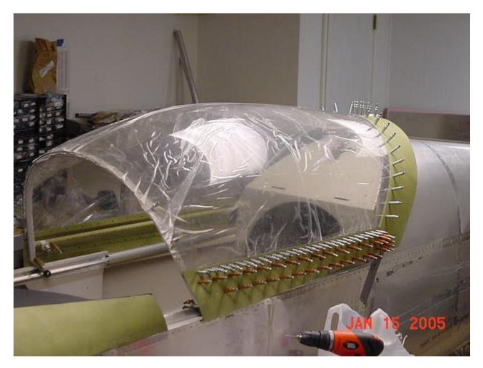
Notice in the pic above that I drilled the lower row for rivets up to #30 (for a #4 rivet). The plans call for just drilling to #40 (for a #3 rivet). I had some mis-matching of the holes, so I decided to step up a size. I could have just drilled a few holes up to #30 and then used "oops" rivets, but decided to just go for the larger rivets altogether. The rivets along the windshield skins are also up-sized to #4 rivets, so the whole row across will be #4's.
