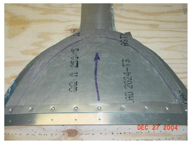
I flipped the parts over face down and line the doubler up just shy of the line I traced under the boot cowl arc and clamped the pieces down. I then back-drilled the arc. Now these pieces are normally bowed and they have to sit together. So I biased my drilling to compensate for the slight bow in the natural shape of the pieces.
